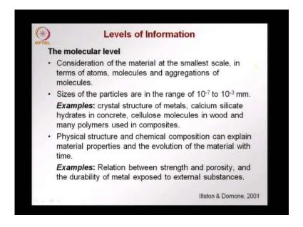
Now why do we need to understands we need to understand this because the physical structure at this scale and the chemical composition gives us an idea of how the material behaves how do we get the material of properties and how this material is evolve with time which is of very high importance when we talked about durable the chemical behavior tells us how durable material, we get ideas about the relations between this strength and the porosity velocities a feature after microstructure.
