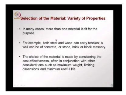
So, in this selection of materials we find that more than one material is fit for a certain purpose for example, when we talk about a tensile element both steel and wood you can carry intension well we saw that the tensile strength of wood is quite good may be not reaching the value of steel, but it is quite high that is reason why in traditional structures we see a lot off ties tensile elements in trusses made.
