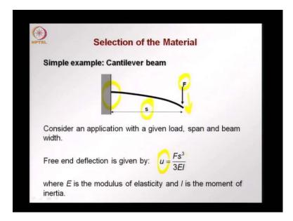
So, we let us take a simple example of a cantilever beam and all of you know what a cantilever beam, it is a beam with a fix tend and it projects out and you have a certain load acting on it. So,
