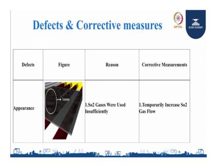
Appearance, reason is So2 gases were used inadequately corrective measure is temporarily increases So2 gas flow and appearance will come in live.
