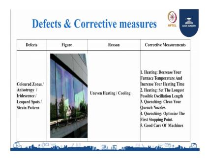
Now, coloured zone leopard spots or strain pattern, reason is simple uneven heating or cooling, decrease your furnace temperature and increase your heating time. Set the
