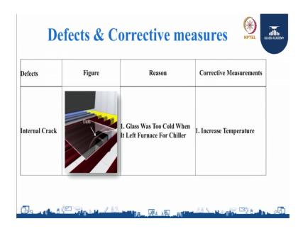
Internal crack, reasons are simple glass was too cold when it left furnace for chiller and corrective measure is increase your temperature.
