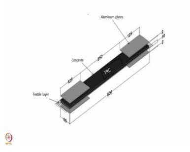
The maximum size of aggregates that we use in this is around 0.6 mm, so it is a very fine grain concrete. So the problem a uni-axial tensile test is the gripping is the primary problem how to grip the specimens. So what we use is a aluminium plates that is attached to the end such that the crushing failure does not happen during the gripping process.
