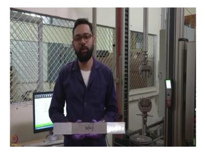
These are specimens that is attached with aluminium plates so we cut out rectangular aluminium plates on the gripping area and we ebbed them or we fix them with epoxy regions and we let them cure for 1 day, then we are doing the test after that. So this prevents the crushing failure of the support due to the pressure that builds up during the testing process or gripping process.
