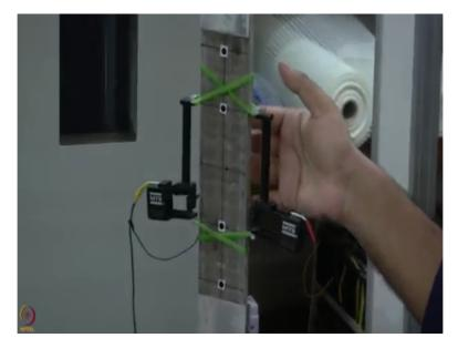
So basically I have marked 4 points or 4 positions in the gauge length of the specimen, the first one is 100 mm gauge length which is equal to the axial extensometer, why? This is to detect whether the video extensometer ratings are as same as that of what we observe in axial extensometer, the second one is a gauge length of 200 mm where (the) that is as per the standards of rilem for testing of textile reinforced concrete.
