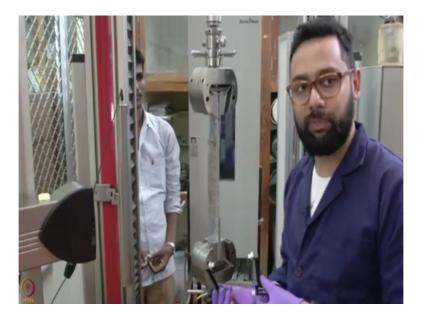
This is a 100 mm axial extensometer so what we are trying to do this is a contact type axial extensometer so we will be attaching the axial extensometer to a 100 mm gauge length on the specimen and this is a dual axial extensometer that means it has two axial extensometers and what we get is average of both the displacement from the two sides, okay. So it (gets) gives you an average displacement that is happening in the two phases of the specimen.
