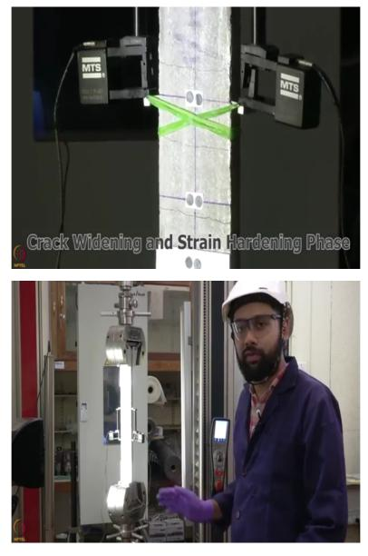
So we will start the experiment you can see the force and the displacement in the you can see multiple cracking forming in the gauge length of the specimen. Now this is where the influence or the advantage where non-contact type video extensometer comes into play, since the cracks can form anywhere, you can also form in the position of an LVDT or a strain gauge. So a non-contact extensometer helps us to take data out even if you have a mechanism like a multiple cracking.
