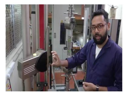
So here is a setup for uni-axial tensile test for TRC, we use two systems for taking out the displacement or the strain of the element one is the axial extensometer, so this is an axial extensometer of 100 mm gauge length as I have said this is a dual axial extensometer where you have two setups for the axial extensometer and you get an average of the two displacement at the two phases.
