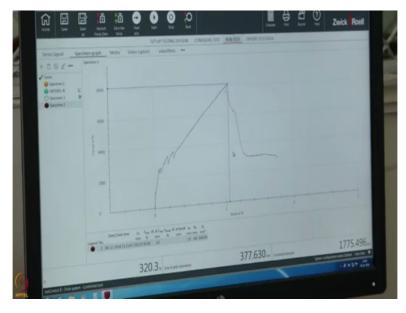
So we have completed the test now and we will look at the stress strain plot of the TRC element and see what are different characteristics that is involved in a TRC element subjected to tensile stress. So this is a basic plot of force versus strain percentage strain we can see two different slopes for the graph, first slope is representative of the matrix properties and the first slope is ended by the first crack formation in the specimen.
