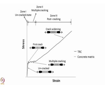
The graph can be basically divided into two segments, the first segment till first crack of the specimen is dominated by the properties of matrix the stiffness is directly proportional to the stiffness of the matrix itself and the second portion is the strain hardening area or the strain hardening zone where the properties of the textile is predominant. Once the multiple cracking has happened then all the tensile stress is taken by the textile.
