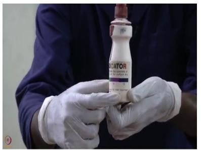
So similarly I will just show how the rainbow indicator performs for measuring the carbonation depth. So this is rainbow indicator where you can see the working range will be 5 to 13. So here the non-carbonated zone will be the violet one. So the carbonation zone which will be expected to have a green color over this surface, so we will just spray this as we did for phenolphthalein indicator and then we will measure the carbonation depth as similar to what we did for phenolphthalein indicator.
