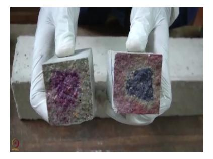
So similarly for concrete specimens we can take slices at each time interval using share cutters and then do the measurements as I did for motor specimens.
