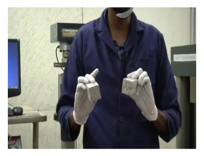
So after the prism is broken, so we are just going to spray the phenolphthalein indicator over this. So this is the freshly broken surface. This kind of breaking is preferable than socket just to avoid the calcium leaching which could possibly occur during the saw cutting, the carbonation front will get disturbed when there is saw cut has been done. And the spraying of the indicator should be done at once to avoid any other external carbonation which could possibly occur.
