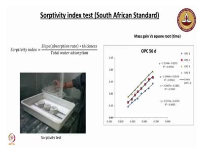
So accordingly you keep measuring the mass of the sample at different time intervals and once you plot the change in mass over time square root of time you take the slope of that curve which will be absorption rate of the moisture inside the sample.
