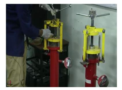
Going forward we will see the next experiment which is on gas permeability, we have seen chloride based test and moisture based test and gas also becomes a very critical factor. For example we can have the carbon di oxide penetrating into the sample, reaching the surface of the steel and start to initiate corrosion. So in these critical conditions you need to assist the quality of concrete by means of its gas penetrability characteristics.
