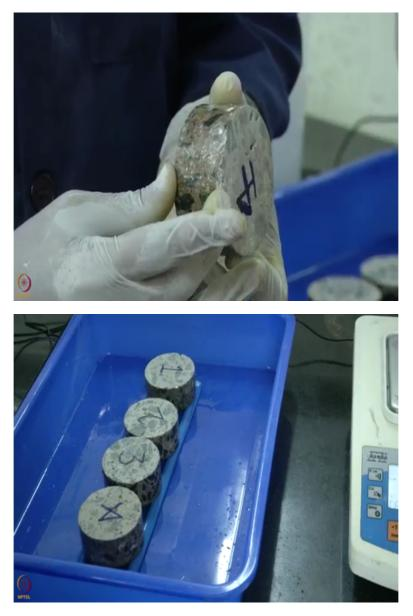
So the next experiment which we are going to see is sorptivity test which is indicative of the water absorption rate in the sample. So depending on concrete structure is being put in place you need to do a different assessment, the first test which we saw on rapid chloride permeability is more dominant parameter when you are trying to measure a structure measure a parameter for a structure put in place of chloride exposure.
