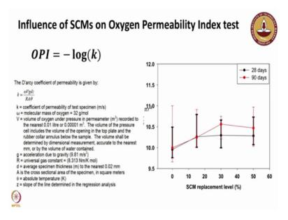
So depending on the mixture proportioning of the concrete or the water cement ratio of the concrete how dense the structure is you will have a difference in the rate at which gas moves
