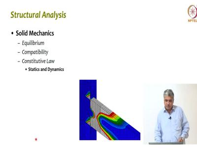
And in this, the fundamentals are the three pillars are equilibrium of forces or stresses compatibility of deformations of strains and of course, constitutive laws or which is you know how materials behave. And behavior is not just under for the given loads, the behavior under statics and dynamic conditions. So, what are these?
