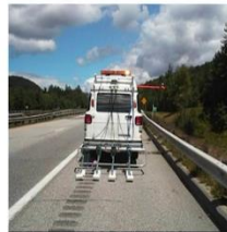
Low speed, high resolution using four 1.5 GHz antennas spaced equal distance apart
