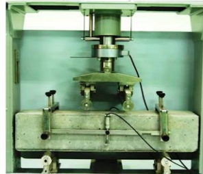
Four-point load test
