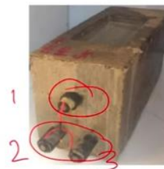
Specimen being exposed to 3% NaCl solution
