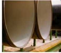
Cement mortar lining of steel pipes for drinking water project
