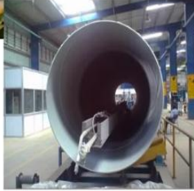
Food Grade Epoxy Coatings of steel pipes for drinking water project
