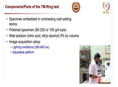
Coming to the test procedure, we have two parts, one is the specimen preparation and second one is the actual test procedure. For the specimen preparation we have a regular steel rebar which is cut into a small piece, this rebar will be polished using sandpapers of different grid sizes ranging between 80 to 220. Once polished we embed the specimen in a cold mounting epoxy which in this case has a contrasting color, this will help at the end when we take the photograph.
