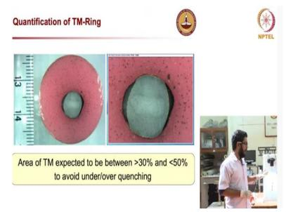
The quantified TM area is expected to be in the range of 30 to 50%, an under quench TMT rebar will have an area of tempered Martensite less than 30% which can result in premature strength failure or corrosion and an over quench case where tempered Martensite is grater than 50% of the area can compromise in ductility.
