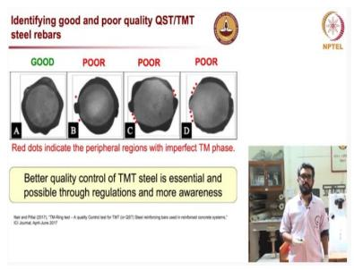
So as shown on the screen the result of this test it would be different cases. Case A is good where you find a completely TM ring and an FP core whereas cases B, C, and D are poor TMT bars where an incomplete TM ring is present, or an eccentric FP core is present. This can have implications on the strength and corrosion characteristics.
