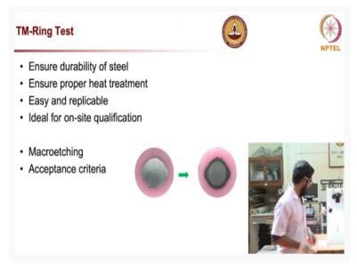
This is where TM rink test comes into picture where it used to ensure the durability of the steel in terms of proper heat treatment. This test is easy and replicable to do on site and it involves macro etching in it. This is more of an enhanced version of macroetching.
