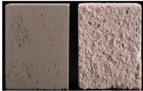
Good resistance by CAC cement Poor resistance by Portland cement
