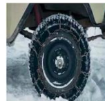
Abrasion on pavements increase due to wheel chains
