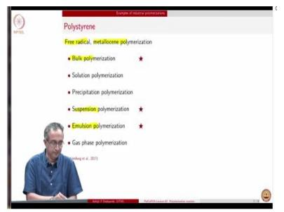
Polystyrene which is also one of the largely produced polymer, it is reaction can be free radical or also metallocene. In fact using metallocene we can also get tactic polymers, in the sense we can control the tacticity we can get syndiotactic or isotactic polystyrene. This was not possible prior to the discovery of metallocene catalyst, so generally therefore polystyrene is used as a commodity polymer.
