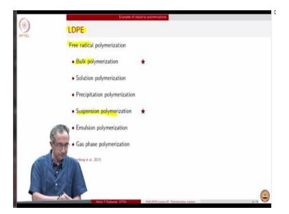
So, let us now survey quickly what are the modes of polymerization which are dominantly used when industrial scale polymers are manufactured. The first example that we will take is the low density polyethylene which is produced in very large quantities. And it is a free radical polymerization mechanism which is used and largely we use bulk polymerization and suspension polymerization for production of this.
