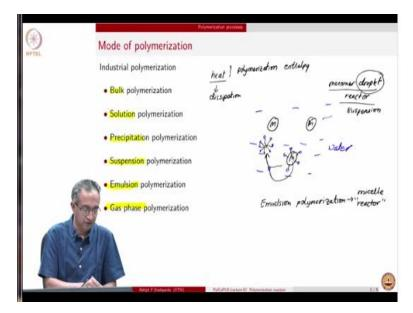
So, largely when we look at the set of polymerization processes which are used in industry they are bulk polymerization or it is also referred to as the mass polymerization. Basically monomer is taken along with initiator; let us say if it is a free radical polymerization. And then reaction is carried on and there is no solvent, there is no other medium, so that is why it is called bulk polymerization.
