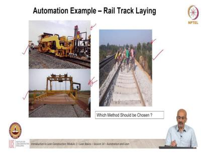
Now coming to this context of automation in India or automation in an emerging nation. So, here is an example, if we look at a track, laying a rail track or even laying the sleepers on a rail track, we have three methods that are followed in our country. We have a highly automated system which is being followed in the freight corridor. We have kind of a mechanized system which is very common in many of our sites. We also have a very manual based system.
