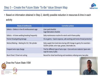
Step 3 is to create the future state to be value stream map. Based on the information obtained in step 2, identify possible reduction in resources and time in each activity and example is given. So, identifying various wastes and bottlenecks, and what are the possible corrective action that you can take in order to mitigate those issues. Based on this information, then you draw a future state map, value stream map, it means what can you achieve by taking care of all these problems,
