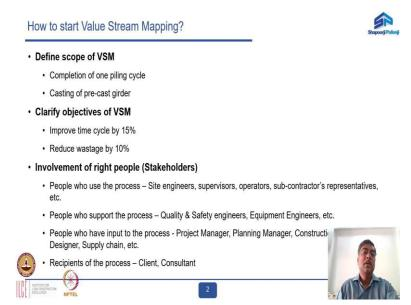
Now, how do we start the value stream mapping on the project? The first and foremost important point is to define scope of value stream mapping. Like an example, you want to do a Value Stream Mapping for completion of one piling cycle. So, we have to focus only on the activities which are involved from start to end of one piling cycle or another example could be casting of precast girder at site.
