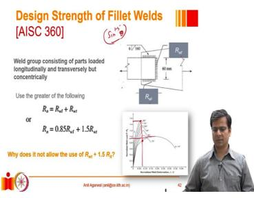
So, the displacement, when the end fillet reaches its full strength, the side fillet only reaches this much of strength which is not really equal to its ultimate strength.
