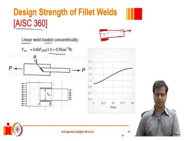
So, they were linear welds loaded concentrically, but it was not a combination of longitudinal and transverse. If we have such a situation, then we cannot use this equation.
