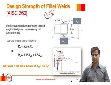
So, when we are taking the ultimate strength of the end fillet, we cannot take the full strength of the side fillet; we have to only take about 85% of the side fillet. However, the other option is to take the full strength of the side fillet.
