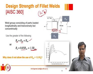
But if you want to do that, you cannot amplify this one also, or you cannot use the full strength of this weld. In fact, you have to reduce the strength of this part by 15% and use only 85% of the strength. So, either you can use both of their full shear strength or for this one, for the end one, you use the full tensile strength, which is after amplifying for the factor, but then you have to reduce the strength which is available at the other weld. The question is, why does it do that?
