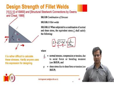
And then, make sure that effective stress, that f\_e that we get remains less than f\_u divided by  $\sqrt{3}$  divided by  $\gamma_{\text{mw}}$ . So, it is basically trying to say is that you calculate the effective stress
