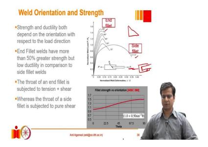
And this angle theta is measured with respect to the direction of loading. So, the direction is in the longitudinal direction. So, basically, this theta represents the angle between the loading and the longitudinal axis of the weld. Then they plotted the deformation on the weld against the load resistance of the weld. And what they observed was quite significant here, which controls the behavior of a fillet weld.
