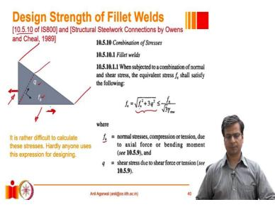
So, we have just seen that for fillet welds, the Indian code recommends using of f\_u divided by  $\sqrt{3}$  as the design stress value or the nominal stress value. And that is what you will use for designing of fillet welds under any type of loading condition. There is also another clause 10.5.10 in IS 800 which also gives a slightly different requirement or equation for designing of fillet welds, especially for the situations where there is a combination of stresses are acting simultaneously.
