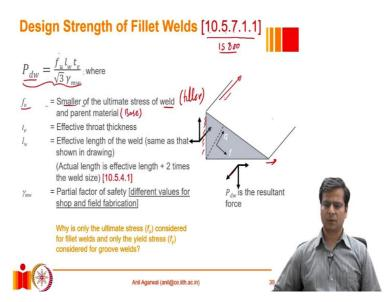
The first component could be in the horizontal direction. The other component could be on the vertical direction. And the third component could be in the longitudinal direction of the weld. So, this is the longitudinal direction of the weld. The third component of that force would be in that direction. And the other boundary of this weld will be resisting all these forces by equal and opposite forces.
