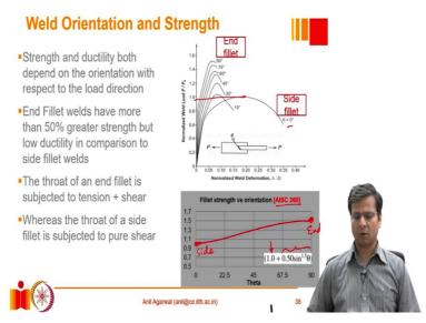
The welds which are side welds which have a 0 smaller angle, they act in a much more ductile manner than the welds that are at the ends. There are various researchers who have also tried to quantify the difference here. The American steel design code AISC 360 actually provides an equation which gives you a relative variation as you change from angle 0 to 90 degree angle.
