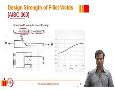
What does the international practice involve? So, internationally, as I had mentioned before, for example, if we take the example of America, in the U.S., the prevalent design code for steel structures is AISC 360. And as we have seen this equation; this equation I believe you have seen already, the second part of this equation. So, what it says is that, this material would have the strength of 0.6 times f u.
