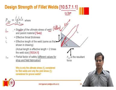
1\_w is the length of the weld in this longitudinal direction. So, that is an obvious thing, because we can expect that, as this is the width of the critical section, there will also be a length component, and together they will form the critical cross-section area.
