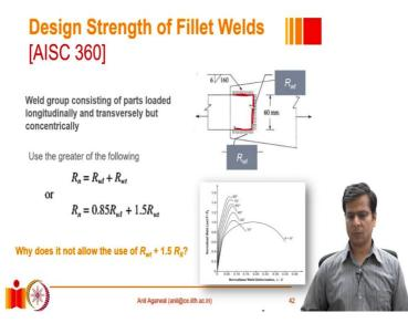
In such a situation, when a portion of the weld is longitudinal and a portion of the weld is transverse in comparison to the direction of loading, which is the case here. So, you have got 2 plates, lap joint, and this is the total weld length. Out of the total length, one portion of it is transverse and the 2 equal and opposite portions are resisting the load longitudinal action. And it is a symmetric weld, the load is concentric in everything.
