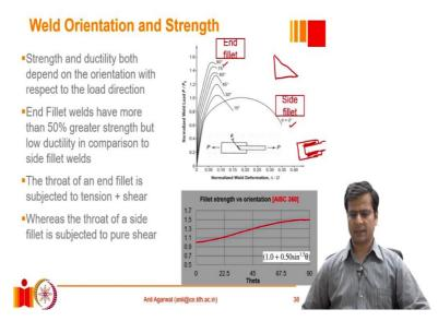
But the other situation that we saw where there was a possibility of tension, a combined tension plus shear, is where it becomes slightly more complex. So, what does it depend on? So, here is a schematic of that experiment that several people have done. They have taken 1 plate and another bar or a plate. They are lap joined together with the help of a fillet at the end.
