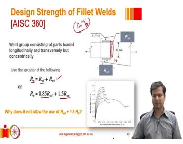
Or what you may do is, you can take, you can increase the strength of this weld by 50%, which is as per that equation which had this function of sine to the power 1.5 theta. Do you remember? So, as per this equation, we were having an amplification of 50%. So, it says you amplify this weld strength by a factor of 50%.
