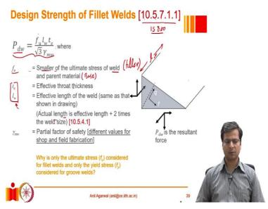
So, we are basically, when we multiply t\_e and l\_w, we are calculating the critical crosssection area. The actual value of the length will be slightly higher than the l\_w value. But as an engineer, we need not worry about the actual length. Whatever we calculate in our design calculations, that is what we will specify in the drawings also.
