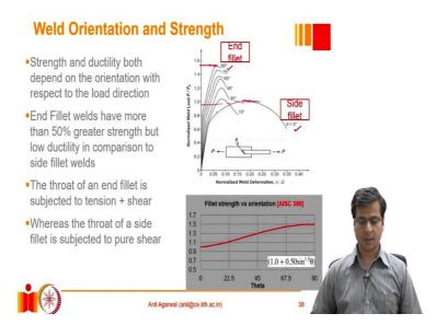
So, we can anticipate that since this is primarily shear behaviour and this is some shear and a significant amount of normal stresses are involved, we can expect that von Mises criteria would also suggest that the shear strength should be smaller than the yield strength or ultimate strength under tension. So, that is understandable. Also the ductility is quite a significant part here.
