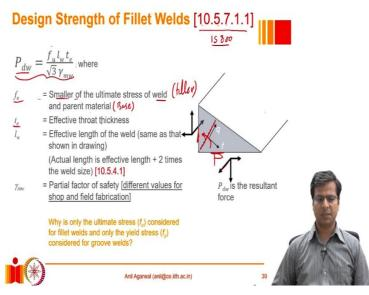
So, of course, that force has to be transferred from here to here, from this edge to this edge, and that has to pass through this interface. And that is why this interface dimension t\_e is adopted. We have already discussed how to calculate t\_e for different types of fillet welds. (Refer Slide Time: 13:16)
