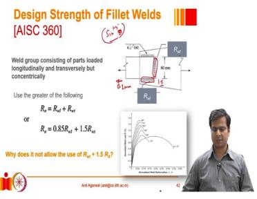
So, if this plate is moved, let us say by a particular displacement, let us say 0.1 millimetre. So, at 0.1 millimetre, maybe the end fillet would have already, would have reached its ultimate strength, but at that time, the side fillet would not have reached its ultimate strength, it might still be at a much lower strength. And if that is the case, we may not be able to utilise the full strength. We can understand that by these plots.
