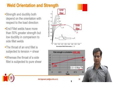
And in between it has this function, sin to the power 1.5 theta that controls the interpolation function.
