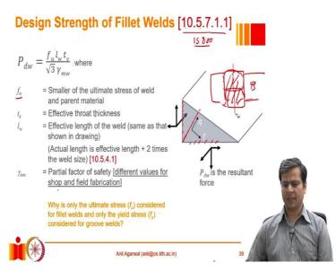
So, for example, in case of a groove weld, when we were talking about a groove weld, we had these 2 plates let us say. And we wanted to weld these 2 plates together using a groove weld. So, when we provide a groove weld, we completely fill this area. And then, the groove weld actually behaves exactly like the plate, the base metal. When it does that, the failure location is not already restricted to a particular plane; it can be anywhere.
