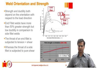
So, let us say I give you a scenario where there is a plate, and there is another plate right under it. The 2 plates are welded together using a fillet weld. And imagine that everything is symmetric and so on, so that there is no moment introduced. Now, what we do is, pull this plate outward, while we push this plate into the screen, into the board. Now, what do you expect the stress state in that fillet would be? In this situation, the stress state is relatively simpler.
