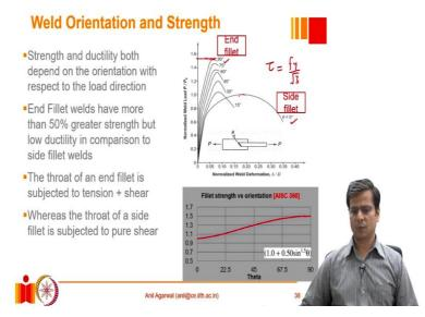
So, when we look at this member, we understand that the behaviour of most of the ductile materials can be predicted by using von Mises failure criterion. If we use von Mises failure criterion, it says that the shear strength is equal to yield strength divided by  $\sqrt{3}$ . That is what the von Mises criteria says.
