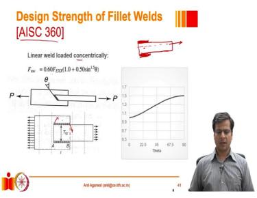
Like the case shown here, the loads are concentric, the welds are symmetric; therefore, the entire force will be going equally to this. And there will not be any moments at the ends which will be acting, which may affect the stress levels. So, if that is true, then we can apply this equation.
