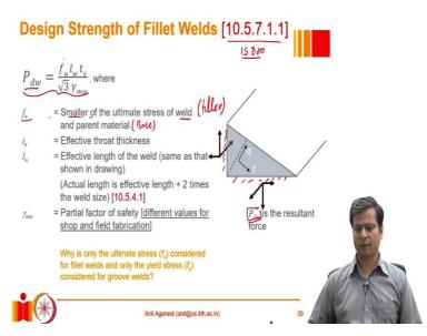
How does the Indian code IS 800 recommend we should design a fillet weld? So, if you go to clause number 10.5.7.1.1, it talks about design strength of fillet welds. And basically, the expression that it gives is P\_dw is equal to  $(f_u \times 1_w \times t_e)/(\sqrt{3} \times \gamma_{mw})$ . There are various terms; let me explain them. f\_u is given by the smaller of the ultimate stress of weld and the parent material.
