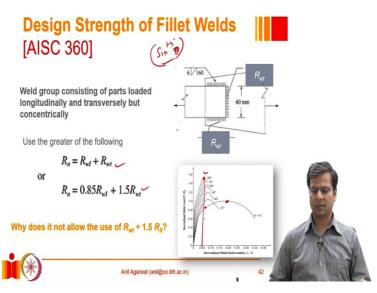
That is the reason either we can use this or we can use this. In fact, we can use greater of the two, because, for the weld to fail, it has to pass both of those peaks, one peak here or one peak here. So, we will consider this peak and we will consider the equivalent force here which lies somewhere here.
