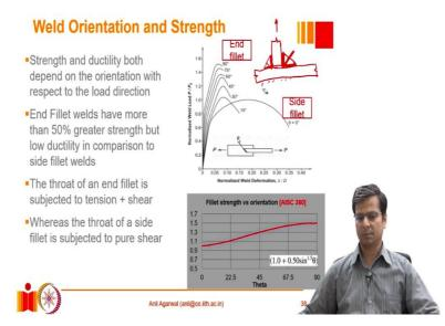
And that is where the; this is the section that would govern the strength of this fillet; same thing here. Now, what is the stress state at this situation at this location? Understanding this is quite complex. Actually, there is a part as we saw, at this edge, it was primarily shear, but at this edge, it was primarily tension. And at this interface, it will be somewhere in between shear and tension.
