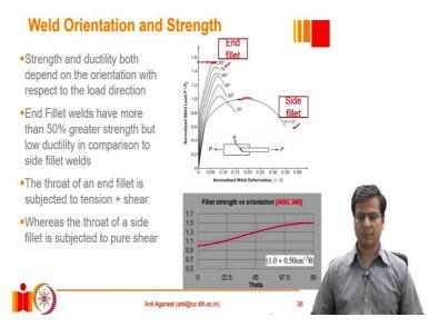
But when the angle changes to 90 degree, that is when we talk about the end fillet, at that time, the strength of that fillet weld is much higher than in the earlier case. That is approximately 50% or higher than the original strength in comparison to the side fillet. Also,
