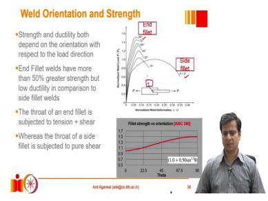
They observed that when we are talking about side fillets where, that is when the angle  $\theta$  is 0, at that time, the strength is very small.
