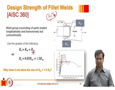
And at the same displacement, what is the force available in the end fillet? And at that time, the end fillet could only have a much smaller strength; it will not have the full strength; it will be only the strength which may be approximately 50% less than the full strength. And therefore, we take only the shear part of it, we do not take the combined amplified part of it. **(Refer Slide Time: 30:20)**
