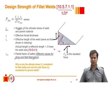
And that makes quite a bit of conservative sense, because a material, a ductile material as we know has the lowest strength in pure shear. Whenever we have a ductile material, if we calculate using von Mises criterion, if we calculate its strength under pure tension or a combination of tension and shear or pure shear, we will see that we will always have the lowest strength under pure shear.
