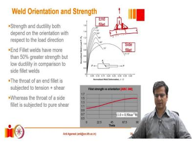
So, actually, the behavior of fillet welds is relatively very different or much more complex in comparison to the behavior of groove welds. The reason for that, as we have discussed in the past also is that the load path for a fillet weld is significantly different from that for a groove weld. So, for example, a fillet weld typically can be approximated to a triangle, a structure of triangular shape.
