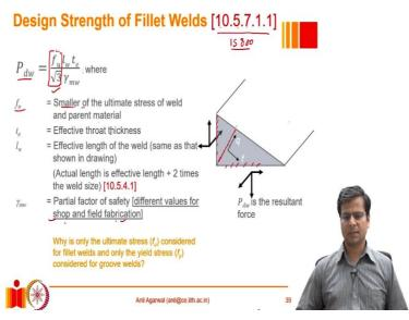
Von Mises criterion basically suggests that if the material has a strength of f\_u in pure tension, it would have a strength of f\_u divided by  $\sqrt{3}$  in pure shear. So, this indicates, this  $\sqrt{3}$  here indicates that we are talking about shear dominated behaviour or failure under shear.
