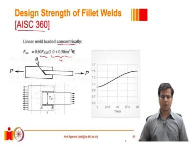
And this is the plot of that second function. Such a situation could be applied to design connections such as these. So, for example, if I have a connection like this, where the load is applied concentrically. That is an important parameter; that is an important condition. Only in these conditions, this equation can be applied.
