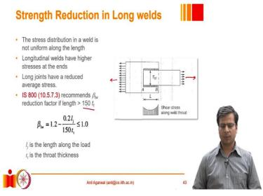
This kind of a situation arises especially when the weld is very long.
