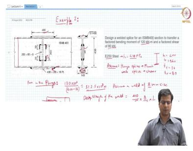
So, now we should do another example again using a fillet weld system. This example, we will see how to design a beam splice. These are all simple connections. So, that is why we are discussing them here. In later chapters, later lectures, we will talk about more complex weld designs where the weld groups act different, resist different types of loads simultaneously. So, here is the problem actually, statement is that we need to design a welded splice for an ISMB 400 section.
