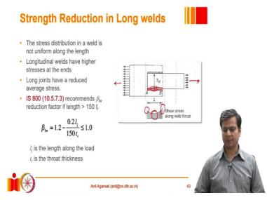
Also there are some challenges when we design welds. There are some other considerations that we have to keep in mind. If we provide a weld which is very long in comparison to its size, then we have to be mindful of the situation, which is shown here through this schematic also. So, here is the lap joint. You are pulling this plate in this direction and restraining the other plate in this direction.
