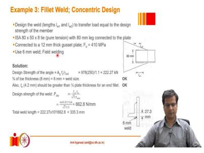
So, let us do one example now on the designing of a fillet weld. So, here is the question. We have got a gusset plate. This is a gusset plate that is connected to an angle by using a number of fillet welds as shown here. So, the total fillet weld is connecting the angle to the gusset plate on 3 sides. The angle dimensions are; it is an IS standard angle of size 80 millimetre by 50 millimetre by 8. So, that is this angle. And this is the gusset plate.
