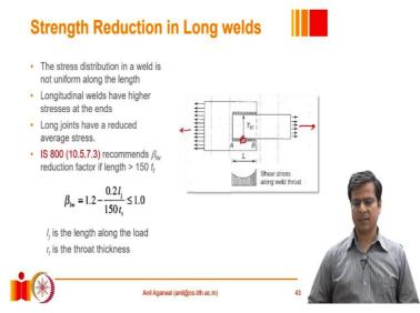
And because of that requirement, we cannot simply take the ultimate strength at any place as the actual strength of the entire weld.
