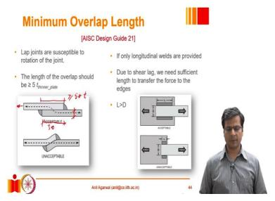
One way to achieve that is to make sure that this length of the overlap that is provided here should be at least greater than or equal to 5 times the thickness of the plate. So, we know the plate thickness. If plate thickness is let us say 6 millimetre, we have to at least apply, make sure that 30 millimetre overlap is available; and larger the overlap, smaller the moment would be.
