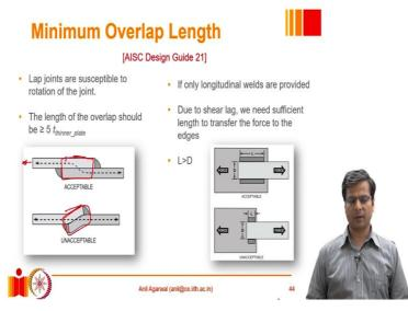
This joint is subjected to a bending moment demand. And there is a possibility that the joint will become more flexible, or it will bend in such a way so that these forces align. And therefore, once these forces would align, the moment demand will disappear. However, we have to prevent such a possibility. We have to make sure that the weld does not have such a large moment demand which can make it bend this way.
