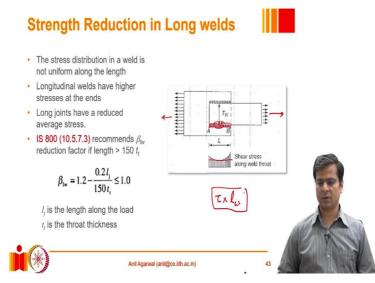
So, if we know that this weld has a particular strength, we cannot simply multiply it with the length of the weld and say that this is the strength of the entire weld, because the stresses will not be uniform, and we have to be careful.
