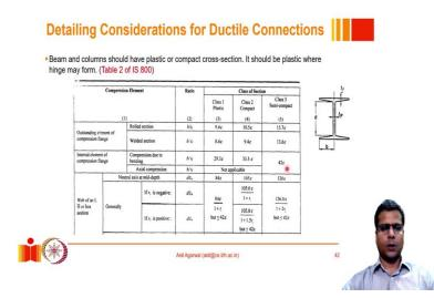
In addition to these there is also there are also a couple of other requirements one such requirement is the use of plastic type of slender cross sections. So, you might recall that whenever we wanted to avoid local buckling of the cross section we were required to use a semi compact or compact cross section based on different provisions. We were never using until we talked about earthquake engineering we never used plastic cross sections we never discussed this column.
