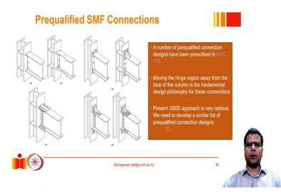
In order for us to know the rotation capacity of a connection presently we have to go to an action F of our IS800 which gives a very cumbersome process and it would be very very difficult for a design engineer to actually be able to calculate the rotation capacity of any given connection design. What American standard AIC358 does is that it prescribes or it provides a list of some pre-qualified special moment registering frame connections.
