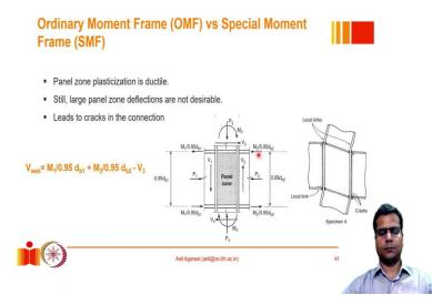
So, when designing a panel zone, we have to calculate the shear force demand on the panel zone and then design it for that kind of a shear force. So, because we want to avoid large panels on deflections for two reasons, a very large deflection in the panel zone will make the column non-straight and create instability in the column that would be very risky for the structure.
