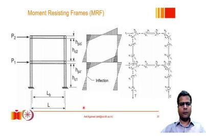
Now in this lecture we will focus primarily on the moment frame resisting systems. And there are two distinct types of movement frame resistance systems one is known as ordinary moment frame resisting moment resting frame the other one is known as special moment registering frame. There is also another variety prevalent in American codes, known as intermediate moment registering frames, but that is not mentioned in the Indian course.
