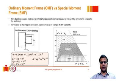
With curves which relate the rotation with moment, there is a limit set according to this equation. So, from various types of connections these equations have been developed and we can actually fit our connections we depending on all the parameters that the connection has we can actually find the values. And then we can find out what my connection's rotation capacity
