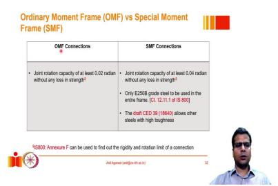
So, as I was talking about an ordinary moment resisting frame versus a special moment resisting frame. So, an ordinary moment resting frame is basically a less that type of rigid connection it is also a rigid connection sometimes even some additive connections are also permitted or rough can also be considered as an ordinary moment resistance member or element.
