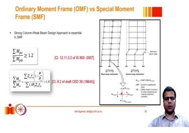
What do we understand by strong column weak beam theory. So, at a joint the idea is that under the earthquake loading the hinges would form but those hinges should not form in the column. So, for example, in this frame at this location, if the hinge has formed in the column that leads to a complete unstability of the structure, then that structure could collapse.
