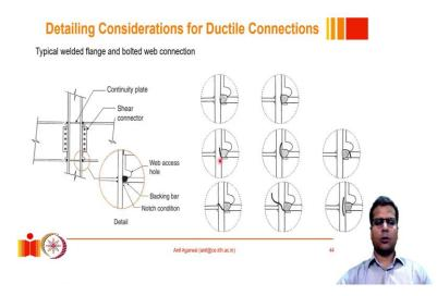
Now we will talk about some of the detailing aspects of rigid connections. So, when we want the rigid connection to be ductile we have to make sure that there are no risks of any fractures or premature fractures to happen in the connection. Wherever we have bolted connections typically fractures can be controlled and we can avoid the moves in which a certain fracture can happen. However welds are relatively unpredictable in comparison to bolts.
