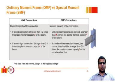
So, as we have just seen, the code requires the existing code IS800 requires the columns to be stronger by more than 20% than the beams. So, columns for moment capacity should be at least 20% greater than the beam's moment capacity, which is true even for an ordinary moment frame. And special moment frame if they are using digit connections however ordinary moment frame allows the use of semi-rigid connections.
