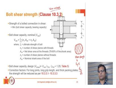
So, instead of using yield stress, we would use ultimate stress,  $f_u$ . But  $f_u$  is the ultimate stress of steel or the bolt material in pure tension condition. In shear condition, the strength will be given by  $f_u$  divided by  $\sqrt{3}$ . Where is this  $\sqrt{3}$  coming from? Do you folks know? What is the reason for a  $\sqrt{3}$  factor for shear? The shear strength of ductile materials is very accurately predicted by a criterion called Von Mises criterion.
