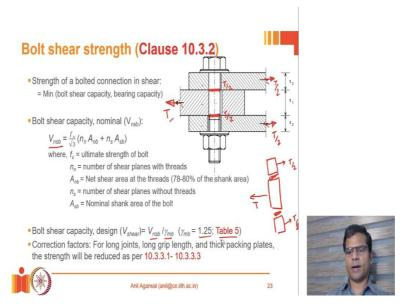
Now, once we know the nominal strength of a bolt in shear, we can divide it with the factor of safety. Now, this factor of safety for a bolted joint in bearing failure or bearing type of a joint is given as 1.25 in Table number 5 of IS 800. So, you go to IS 800, go to Table number 5, you will find the value of  $\gamma_{mb}$ , which is basically the material factor of safety for bolted joints.
