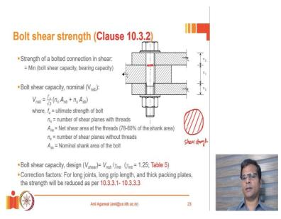
So, when the bolt is subjected to shear force, you can imagine that this is circular surface, a circular round surface which is subjected to shear force demand. And the shear strength of that surface would be actually given by the ultimate stress in shear multiplied by the cross-section area. So, if this is the cross-section area of the bolt, we will take this cross-section area multiplied by the shear strength.
