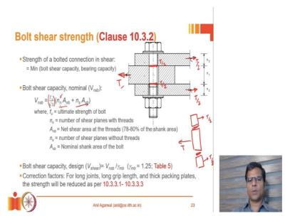
This is the middle portion; I am pulling it by force T. Then this is the other portion which is being pulled by T divided by 2. This is the other portion which is being pulled by T divided by 2. So, how much is the force demand at this shear plane? It will be equal to T divided by 2 at each plane. Each of these two planes will be subjected to a shear force demand of T divided by 2.
