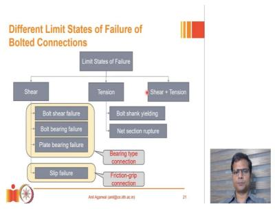
Now, we will talk about the actual design process for a bolted connection. So, first, in this chapter, we will basically study how to design a single bolt. And the bolt group design basically, we will do towards the third section of this course. So, first, before we design a bolt, we have to understand what are the different ways a bolt can fail. So, the ways are also known as limit states of failure.
