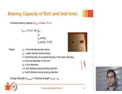
Before we get into the other factors, let us also talk about the bearing type of a failure. So, you might remember, the first limit state was the bolt shear failure and the other two limit states were bolt bearing failure and plate bearing failure. So, as we had seen, if a bolted joint, if a hole is subjected to a shearing stress, it actually translates into the bearing stress concentration at the bolt hole surface.
