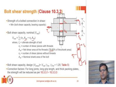
Now,  $A_s$  is easy to calculate. If we know the diameter of the bolt, we can calculate the crosssection area of the bolt. That is the cross-section area of the shank.  $A_n$  can be calculated as by assuming that the net cross-section area is approximately 78 to 80% of the shank area. So, I hope all the required inputs are available here.
