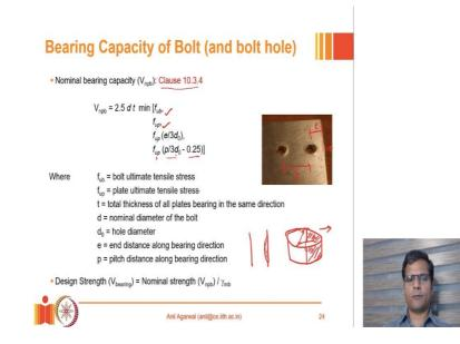
The expression for the bearing strength of a bolt is given in clause number 10.3.4 of IS 800. Now, here, as you might imagine, if I look at a bolt hole and there is a shank inside, there is a bolt inside which is loading this half of the cross-section or this half of the shank surface area in this direction. Now, basically the parameter that should play a role here is the thickness of the plate, the diameter of the bolt.
