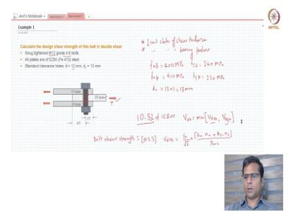
So, we had just gone through the 2 limit states for bolt failure. One limit state was for the bolts which are subjected to shear and are bearing type. There are 2 limit states. One limit state was limit state of shear failure, and the other one was limit state of bearing failure. So, let us do one example here. Here you can read the example. It is required to calculate the design shear strength of this bolt in double shear.
