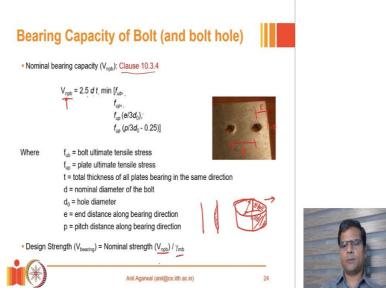
So, and then, basically depending on whichever factor of the 4 of these governs the capacity, which will be the smallest of the 4. The smallest of the 4 will govern the capacity. So, we will calculate all these 4 factors; we will take the smallest of the 4. And that multiplied by t multiplied by d multiplied by 2.5 gives us the bearing strength of the bolt in bearing. And again, the design strength; so, this will be the nominal strength; n stands for nominal strength in
