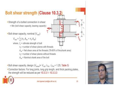
Now, if the total force is T, and let us say this is divided equally between the 2 layers, because these thicknesses are equal. So, this will be T divided by 2; this will be T divided by 2. And if that is the case, the force demand on each shear plane; these are the 2 shear planes I have marked here. The force demand on each of these shear planes will be how much? Take a moment to think about it.
