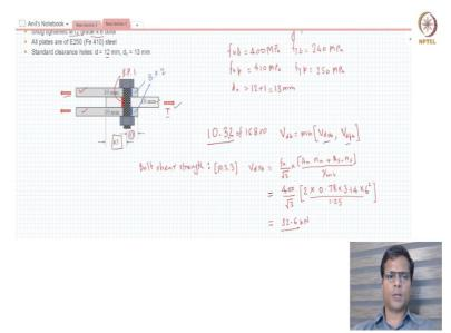
Now, we know that gamma mb is actually equal to; by the way, this is for 1 shear plane. For the 2 shear planes, it will be equal to; since there are 2 shear planes, it will be equal to summation of the 2 strengths. So, first we will look at  $f_u$ , that is 400; we know  $f_u$  of the bolt is 400 divided by  $\sqrt{3}$  . Then, we know that there are 2 shear planes. Now, we do not know exactly what is the length of the threaded portion and what is the length of the shank length.
