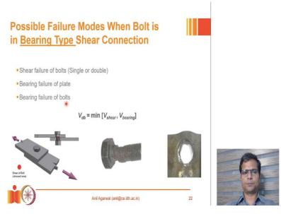
So, if it is a bearing type connection bolt and then it is subjected to shear, there are 2 or 3 distinct ways in which it can fail. So, here is a simple configuration which is shown to you, where these are the 2 plates which are joined together with a bolt like this. And then, these plates are pulled apart as shown here. And there is a possibility that because of this shear force that is applied on the bolt, the net section of the bolt cross-section can fail in shear or rupture in shear.
