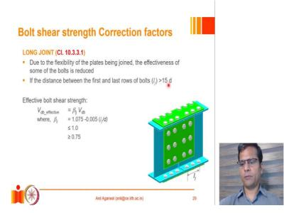
So, let us take a look of a possibility when the joint is longer than a certain limit. So, here I am showing you an example where 2 beams or 2 I sections, they are spliced together using this bolted joint. And I am looking at these 3 bolts which are forming a joint together. Now, if you want to calculate the strength of each of these bolts depending on the length of this joint, the force distribution to each of these bolts may not be uniform.
