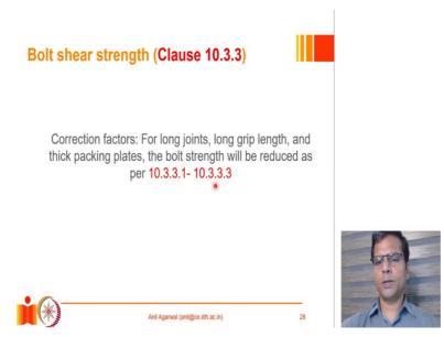
So, now, we will talk about some correction factors. So, as we have already discussed, the shear strength of a bolt and bearing strength of a bolt. However, there are certain conditions under which the full bearing strength or the shear strength of a bolt cannot be utilised. Some of those conditions are listed here. So, for example, if the joint is relatively long, what does that mean?
