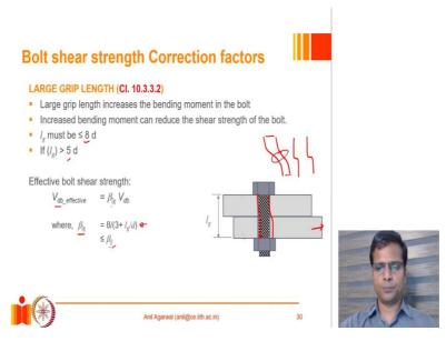
Other aspect or other correction factor that is relevant here is the bolt length. So, if the grip length or bolt length is more than a certain limit, then also the effectiveness of the bolt is reduced. So, here I am showing you an example, in this particular case, this bolt is holding these 2 plates together. Now, when this plate is pulled, this bolt will be undergoing a deformation like this.
