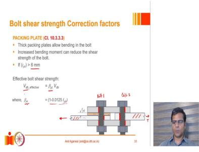
The third important factor here or correction factor here is the factor which accounts for packing plate. So, what is a packing plate, first we need to understand. So, you look at this example here, in this diagram, what you can see here is that there is 1 plate here and there is another plate here. These 2 plates are actually supposed to be spliced by using this joint. So, this plate, let us imagine a situation where this plate is in tension in this direction.
