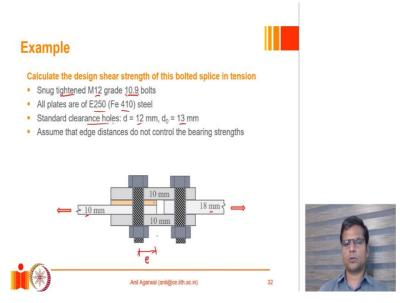
So, now, we have seen these 3 correction factors and we have also seen how to calculate the shear strength and bearing strength of a bolted joint. So, let us do 1 example. We will take the same example that we were working with before with some minor changes. So, let us calculate the design shear strength of this bolted splice in tension. This is a bolted splice. Bolt plate is 18 millimetre; the other plate is 10 millimetre in thickness; it is being pulled in tension.
