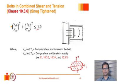
So, as you might see in this diagram, these bolts are likely to be subjected to a combination of shear force because of this force. Direct effect of this force will be a shear force demand on these bolts. And as a result of this moment, there will be tension force demand in the top bolt and there will be some kind of a reduced tension force demand in the bottom bolt most probably if there is a contact between the bottom flange and the column.
