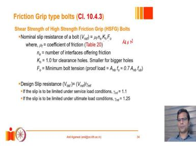
So, since we know that the plates are held in place through friction, the strength of that connection would be basically a function of the friction force. So, the slip resistance of the bolt will basically control the strength of the connection. So, a single bolt would have a strength which is basically equal to the slip resistance of the bolt that again can be calculated as the friction coefficient between the plates multiplied by n e.
