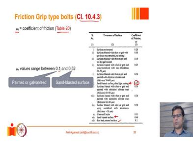
The friction coefficient that we just saw, we can get the values of friction coefficient from table 20; this is again clause 10.4.3 of IS 800. The values of friction coefficient between the 2 steel plates can vary between 0.1 and 0.52. So, this is a wide range and of course it depends on the surface treatment that is provided between the 2 plates. So, if the 2 plates are treated with a smooth finish; what could be an example of a smooth finish?
