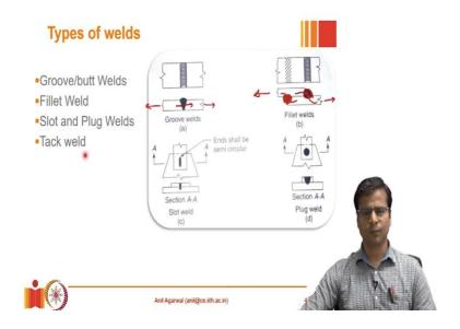
In typical structural applications, geometry wise we can classify welds into these 4 categories. The first one is the groove weld, also known as butt weld. So, here you can see some examples of a groove weld. These are the 2 plates of equal thicknesses. They need to be equal thicknesses. Here is just an example. So, if these 2 plates are to be joined using a groove weld, basically we fill the gap between the plates with a weld.
