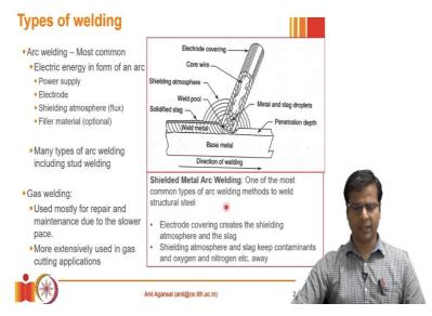
Welding is a very common technique of joining structural steel members, which is used very frequently in construction. The most common type of welding is the one which uses electricity, that is known as arc welding. And the other one which is relatively less used is gas welding. This is more frequently used for cutting operations in comparison to regular structure and steel welding.
