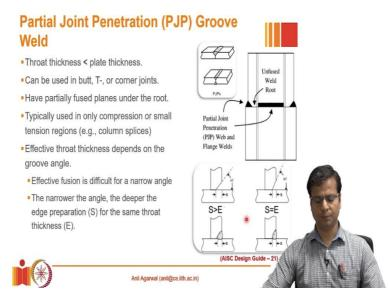
The other variety of groove weld is known as partial joint penetration weld. In case of a partial joint penetration weld, only a fraction of the total thickness of the plate is fused and the rest of the thickness remains unfused. It again can be used in various configurations including a butt joint, a T-joint or a corner joint as we saw before.
