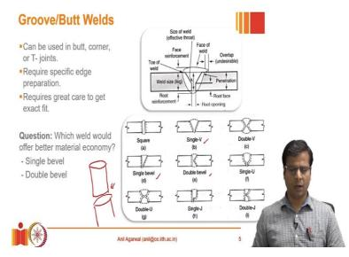
Let us discuss groove welds first in some more detail. So, as we had seen, groove weld is also known as butt weld in common language. So, basically, if we have these 2 plates that we want to join together, the easy option is just to have a groove in between and fill it with filler material. Now, the groove can be just the gap between the 2 plates and we do not have to create this kind of an inclined groove.
