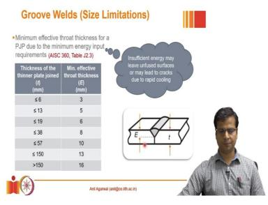
When it comes to the size of a PJP, that is Partially Joint Penetration groove weld, sometimes we of course have to provide the joint, the weld of sufficient size, so that it has the ability to resist the design loads, whatever the loads are coming; but sometimes, the load requirement may be very small and we may require very small amount of joint. But there are other considerations which force us to put a minimum weld size as per this clause here.
