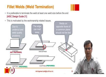
As a designer we should be mindful of this fact that terminating a weld can be a critical factor in the overall performance of a structure. So, generally it is not preferable to terminate a weld that is the end of a weld being located at a position where there is already a perpendicular edge. So, for example between these two options here you can see there is a horizontal plate in both cases and there is a vertical plate which is being fillet welded with each other.
