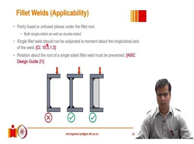
As we just discussed the fillet welds behave somewhat similar fashion as the partial joint penetration welds. So, fillet welds since they provide a welding between two perpendicular surfaces and there is always a portion of the combined surface which is not fused together and whether the welding is done on one side or whether it is done on the two sides in both cases there will always be some portion of the surface which will not be fused together and that is where the cracks can start.
