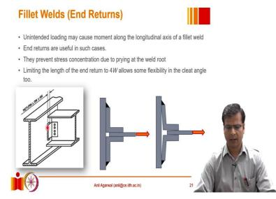
There are however some situations where we may actually want to not terminate the weld right before the end but continue the weld slightly further and then terminate it such a situation is called an end return and an end return. This end return type of a weld is particularly useful in such scenarios here I am showing you through an example. Let us say the same weld that in this connection you may see there is a beam which is connected to a girder and this connection is through a cleat angle.
