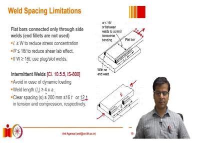
There are also some requirements about the placing of the welds in terms of how far apart the welds can be in the direction of the load, in the direction perpendicular to the load and so on. So, here is an example of two plates that are being fillet welded together through a lap joint. So, this is a flat plate it does not have any angle or anything any protruding part outside and if it is subjected to a tension force demand there are a couple of requirements for it.
