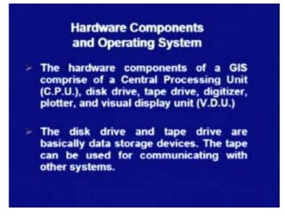
The hardware components of a GIS comprise of a central processing unit; in short we call it as the CPU, a disk drive, a tape drive, a digitizer, plotter and a visual display unit, in short we call it as VDU. The disk drive and the tape drives are basically data storage devices. The data can be used for communicating with the other systems. The disk drive and the tape drives are basically data storage devices. The tape can be used for communication with other systems.
