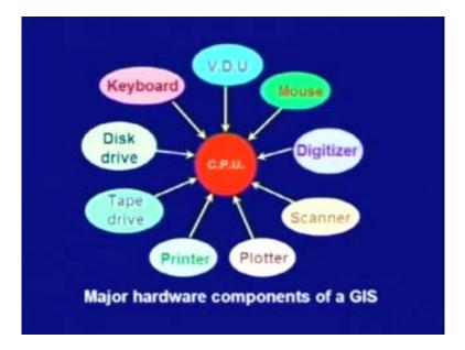
Now, let us look at the graphical display of the major hardware components that we need in a GIS. The core of the GIS is a CPU system which will have a video display unit. A mouse for interactively displaying, interactively sending commands. A digitizer for sending an input data
