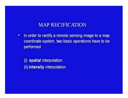
In order to rectify a remote sensing image to a map coordinate system, 2 basic operations have to be performed. First is spatial interpolation and second is intensity interpolation.
