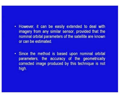
However, it can be easily extended to deal with imageries with similar sensor provided that the nominal orbital parameters of the satellite are known or can be estimated. Since, the method is based on the nominal orbital parameters, the accuracy of the geometrically corrected image produced by this technique is not high. (Refer Slide Time: 18:48)
