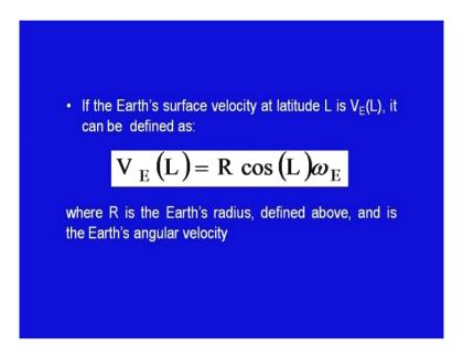
If the earth's velocity at the latitude L is given by  $V_E(L)$ , it can be defined as  $V_E$  equal to R cos of L omega E, where r is the earth's radius defined above and omega is the earth's angular velocity.
