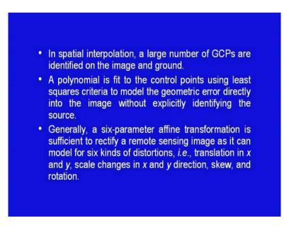
In spatial interpolation, a large of number of GCPs are defined on the image and on the ground. A polynomial is fitted to the control points using least squares criteria to model the geometric error directly into the image without explicitly defining or identifying their source.
