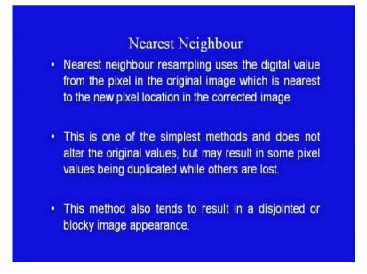
So, let us look at the first method that is nearest neighbourhood. Nearest neighbourhood resampling uses the digital value from the pixel in the original image which is nearest to the new pixel location in the corrected image. This is one of the simplest methods and does not alter the original values but may result in some pixel values being duplicated while others are lost. This method also tends to result in a disjointed or blocky image appearance. (Refer Slide Time: 35:34)
