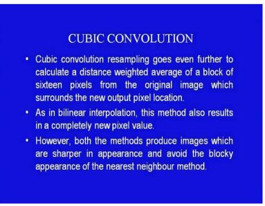
The next, the third method which is cubic convolution, it even goes one step further to calculate the distance weighted average of a block of 16 pixels from the original image which surrounds the new output pixel location. As in bilinear interpolation, this method also results in a completely new pixel value.
