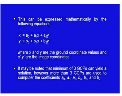
Thus, this can be expressed mathematically by following equations; x dash is equal to  $a_0$  plus  $a_1x$  plus  $a_2y$  and y dash is equal to  $b_0$  plus  $b_1x$  plus  $b_2y$ , where x and y are the ground coordinates values and the x dash and y dash are the image coordinate values. It may be noted that minimum of 3 GCPs can yield a solution. However, more than 3 GCPs are used to compute the coefficients;  $a_0$ ,  $a_1$ ,  $a_2$ ,  $b_0$ ,  $b_1$  and  $b_2$ .
