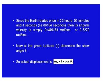
Since, the earth rotates once in 23 hours, 56 minutes and 4 seconds that is 86,164 seconds, then its angular velocity is simply 2 pi divided by 86,164 radians per second or this is equal to 0.7279 radians per seconds. Given the latitude L, now we can determine this skew angle theta. So, the actual displacement is omega zero multiplied by t into cost theta.
