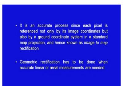
It is an accurate process, since each pixel is referenced not only by its image coordinate but also by its ground coordinate system in a standard map rejection and hence, it is known image to map rectification. Geometric rectification has to be done when linear accurate linear or areal measurements are needed.
