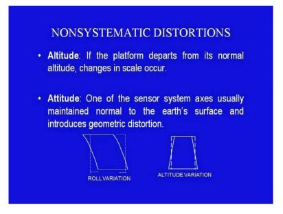
Now, we come to the non systematic distortions which are there. First is altitude. If the platform departs from its normal altitude; it changes, a changes in scale occurs. Next is attitude. One of the sensor systems is usually maintained normally to the earth's surface and introduces geometric distortion.
