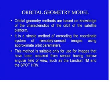
So now, let us look at the orbital geometry model. Orbital geometry methods are based on knowledge of the characteristics of the orbit of the satellite platform. It is a simple method of correcting the coordinate system of the remotely-sensed images using approximate orbit parameters. This method is suitable only for use for images that have been acquired from sensor having narrow angular field of view such as the LANDSAT TM and the SPOT HRV.
