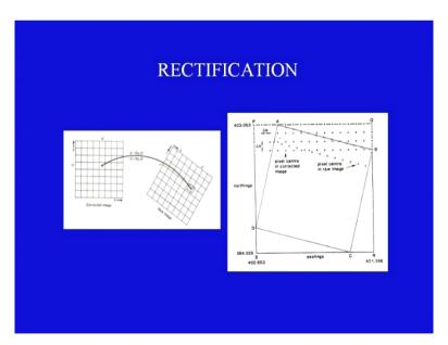
In this particular slide, it illustrates the procedure of rectification which actually has to be carried out. On the left hand side, we can see that there is one image which is tilted which is the raw data and the upright corrected image is shown on the right hand side and we have to map, we have to correct the tilted shape of the image onto the upright corrected shape as shown.
