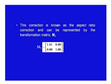
This correction is known as the aspect ratio correction and can be represented by the transformation matrix  $M_1$  where  $M_1$  can be defined to have 2 rows by 2 columns and the elements are as shown in the equation.
