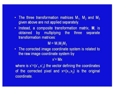
The 3 transformation matrices;  $M_1$ ,  $M_2$  and  $M_3$  are not applied separately. Instead, a composite transformation matrix M is obtained by multiplying the 3 separate transformation matrices. The corrected image coordinate system is related to the raw image coordinate system by x dash is equal to Mx, where x dash is nothing but  $x_1$ ,  $x_2$ , the vector defining the coordinates of the corrected pixel and x is equal to  $x_1$  and  $x_2$  is the original coordinate.
