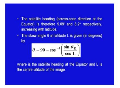
The satellite heading that is across-scan direction at the equator is therefore 9.09 degree and 8.2 degrees respectively, increasing with latitude. The skew angle theta at latitude L can be expressed as theta is equal to 90 minus cos inverse of the ratio of sin theta E over cos L, where L is e is the satellite heading at the equator and L is the centre latitude of the image.
