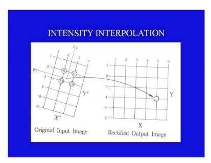
This particular figure shows the concept of nearest neighbourhood intensity interpolation, wherein, on the left hand side we have the original input image and on the right hand side we have the rectified output image.
