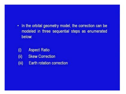
In orbital geometry model, the correction can be modelled in 3 sequential steps as enumerated below. First is aspect ratio, second is skew correction and third is earth rotation correction.
