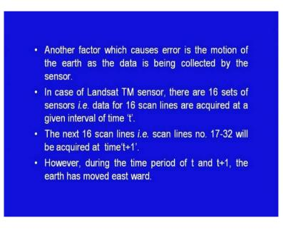
Another factor which causes error is the motion of the earth as the data is being collected by the sensors. In case of LANDSAT TM sensor, there are 16 sensors. That is data for 16 scan lines are acquired at a given interval of time t. The next 16 scan lines, that is scan lines number -17 - 32 will be acquired at time t plus 1. However, during the time period, t and t plus 1; the earth has moved east wards.
