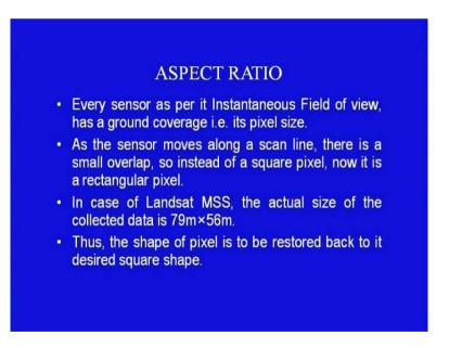
Aspect ratio: Each sensor as per its instantaneous field of view has a ground coverage which is known its pixel size. As the sensor moves along its scan line, there is a small overlap. So, instead of a square pixel, it is now a rectangular pixel. In case of LANDSAT MSS, the actual size of the collected data is 79 metres by 56 metres against the design value of 79 metres by 79 metres. Thus, the shape of the pixel is to be restored back to its desired square shape.
