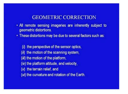
Having done the radiometry correction, now the geometric corrections have to be performed. It has been observed that all remote sensing imageries are inherently subjected to geometric distortions. Such distortions may be due to several factors such as the perspective of the sensor optics, the motion of the scanning system, the motion of the platform, the platform altitude and velocity, the terrain relief and the curvature and rotation of the earth.
