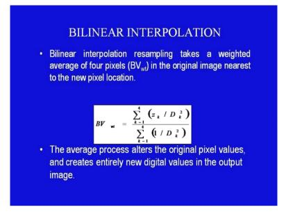
Then, we come to the bilinear interpolation. Bilinear interpolation re-sampling takes a weighted average of all the 4 pixel in the original image nearest to the pixel location. That is as seen in the previous slide, wherein, a graphical depiction of the location of the rectified pixel and the 4 nearest pixel lying in the close vicinity has been shown.
