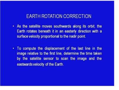
Next, we come to the earth's rotation correction. As satellite moves southwards along its orbit, the earth rotates beneath an easterly direction with a surface velocity proportional to the nadir point. To compute the displacement of the last line in the image relative to the first line, we have to determine the time taken by the satellite sensor to scan the image and the eastward velocity of the earth.
