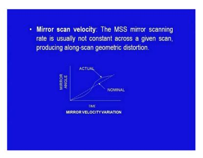
The mirror scanning rate is usually not constant across given scan and produces along-scan geometric distortion. The figure below shows the actual path of the mirror with mirror angle against the calibrated motion path. It may be noted that this type of error probably is no more applicable in the current sensor technology which is being used which is charge couple devices. The earlier mss sensors which carried a mirror type of scanning procedure, this type of error were had to be accounted for.
