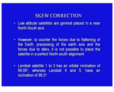
Next, we come to skew correction. Low altitude satellites are generally placed in a northsouth axis. However, to counter the forces due to flattening of the earth, precessing of the earth axis and the forces due to the stars, it is not possible to place the satellite in a perfect north south alignment. LANDSAT 1 to 3 has an orbital inclination of 99.09 degrees; whereas, LANDSAT 4 and 5 have an inclination of 98.2 degrees. (Refer Slide Time: 20:56)
