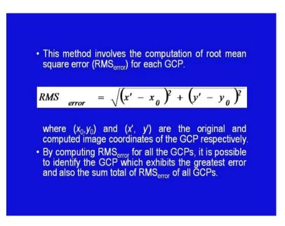
This method involves the computation of root means square error for each GCPs, where the root RMS  $_{error}$  can be expressed as under root of x dash minus  $x_0$  whole square plus y dash minus  $y_0$  whole square, where  $x_0 y_0$  and x dash and y dash are the original and the computed image coordinates of the GCP respectively.
