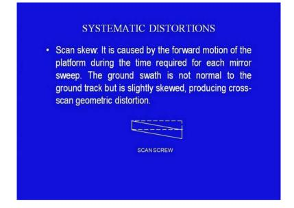
In systematic errors; first, let us look at scan skew. It is caused by the forward motion of the platform during the time required for each mirror sweep. The ground swath is not normal to the ground track but is slightly skewed producing cross scan geometric distortion. The figure below conceptualises the scan skew distortion.
