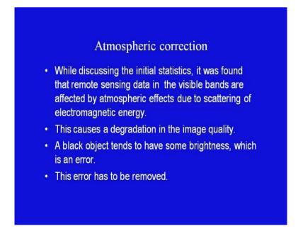
While discussing the initial statistics, it was found that remote sensing data in the visible bands are affected by atmospheric effects due to scattering of the electromagnetic energy. This causes degradation in the image quality. A black object tends to have some brightness which is an error. Now, this error has to be removed. So, let us look at how this can be performed.
