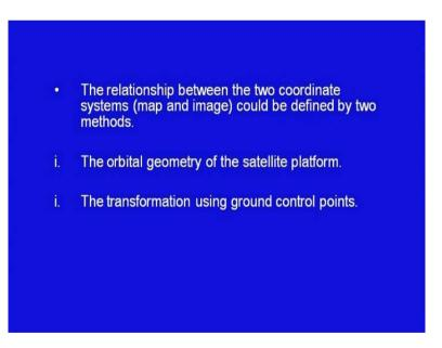
The relationship between the 2 coordinate systems - map and image, could be defined by 2 methods. First, the orbital geometry of the satellite platform and the second is the transformation using ground control points or in short known as GCPs.
