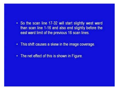
So, the scan line 17 - 32 will start slightly westward than the scan line 1-16 and also ends slightly before the eastward limit of the previous 16 scan lines. This causes a skew in the image coverage. The net effect of this is shown in this particular figure.
