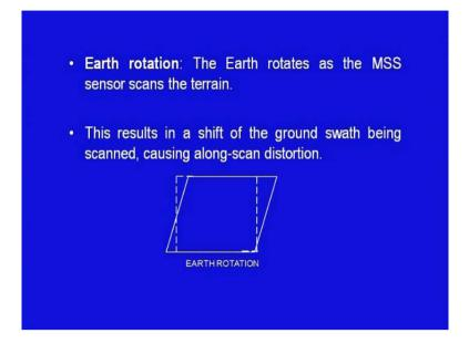
Next is earth rotation. The earth rotates as the sensor scans the ground. This results in a shift of the ground swath being scanned causing along-scan distortion.
