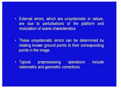
External errors which are unsystematic in nature are due to perturbations of the platform and modulation of scene characteristics. These unsystematic errors can be determined by relating known ground points to their corresponding points in the image. Typical preprocessing operations include radiometric and geometric corrections.
