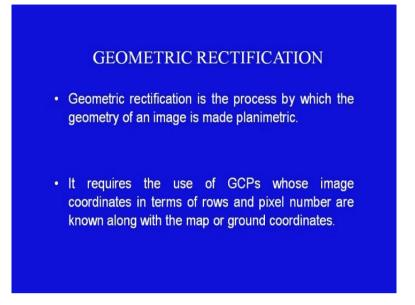
Geometric rectification is the process by which the geometry of an image is made planimetric. It requires the use of the GCPs whose image coordinate in terms of rows and pixel number are known along with the map or ground coordinates.
