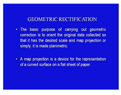
The basic purpose of carrying out geometric correction is to orient the original data collected so that it has the desired scale and map projection or simply we can say; it is made planimetric. A map projection is a device for the representation of a curved surface on a flat sheet of paper.
