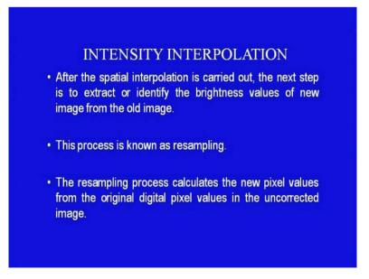
So, now let us look at the intensity interpolation. After the special is carried out, the next step to extract or identify the brightness value of the new image from the old image. This process is known as re-sampling. The re-sampling process calculates the new pixel values from the original digital pixel values in the uncorrected image.
