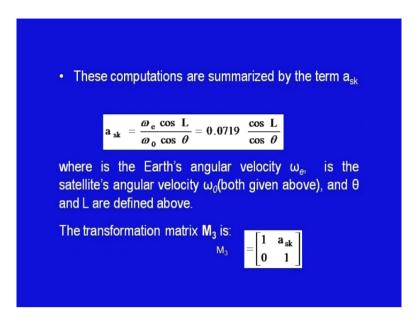
These computation are summarized by the term  $a_{sk}$  which is can be simplified and written as 0.0719 multiplied by the ratio of cos L of and cos theta, where the earth's angular velocity is omega e is the satellites angular velocity omega zero and theta and L are as defined above. So, the transformation matrix 3, can now be expressed as it is shown in at the bottom.
