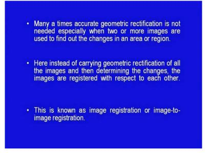
Many a times, accurate geometrical rectification is not needed; specifically, when two or more images are used to find out the changes in an area or region. Here, instead of carrying geometric rectification of all the images and then determining the changes, the images are registered with respect to each other. This is known as image registration or image-to-image registration.
