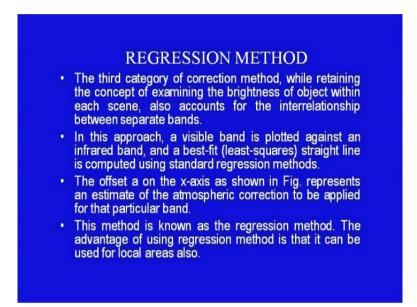
The third method which is regression method of correcting the atmospheric effects, tries to retain the concept of examining the brightness of each object within each scene and also accounts for the interrelationship between the bands. In this approach, a visible band is plotted against an infrared band and a best-fit that is least-square straight line is computed using standard regression methods.
