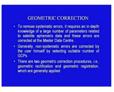
To remove systematic errors, it requires an in depth knowledge of a large number of parameters related to the satellite ephemeris data and these errors are corrected at the master data centre. Generally, non systematic errors are corrected by user himself by selecting suitable number of GCPs. There are two geometric correction procedures that is geometric rectification and geometric registration which are generally applied.
