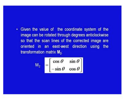
Given the value of the coordinate system of the image can be rotated through degrees anticlockwise so that the scan lines of the corrected images are oriented in an east-west direction using the transformation matrix  $M_2$ , where  $M_2$  can be represented as the matrix as seen here.
