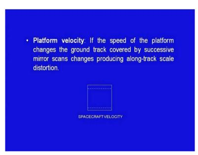
Next is platform velocity. If the speed of the platform changes, the ground tracks coverage by successive mirror scan changes producing a long track scale distortion.
