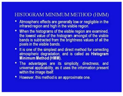
As we have already seen; atmospheric effects are generally low or negligible in the infrared region and high in the visible region. When the histograms of the visible region are examined, the lowest value of the histogram amongst the visible bands is subtracted from the brightness values of all the pixels in the visible bands.
