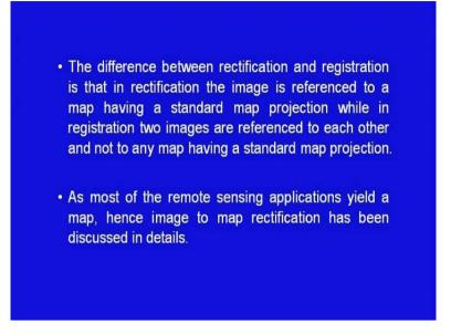
The difference between rectification and registration is that in rectification, the image is referenced to a map having a standard map projection; while in registration, 2 images are referenced to each other and do not have any map having a standard map projection. As most of the remote sensing applications yield a map, hence image to map rectification has been discussed in details.
