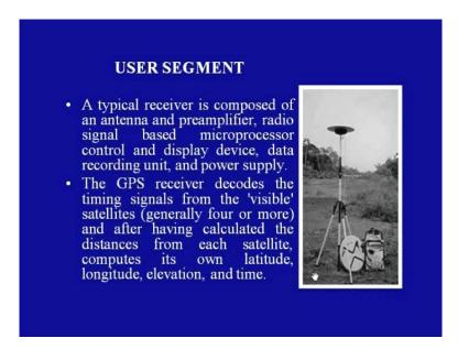
The next slide shows a view of the GPS receiver which is there. We can see that a typical GPS receiver is composed of an an10na and a preamplifier, radio signal based microprocessor control and display device, data recording unit and power supply.
