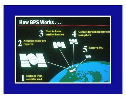
This slide shows the 5 logically steps which are there. First of all, we find the distance from the satellites which are used. In order to find out the distance, we need to find what is the time required by the signal to travel from the satellite to the point on the earth. Thus, the second step is we require accurate clocks.
