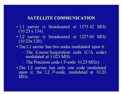
When we look at the signals which are being broadcasted by the satellite; first, carrier wave L1, it broadcasts at a frequency of 1575.42 mega hertz which is 154 times the fundamental frequency of 10.23 mega hertz which has been generated by a very precise atomic clock.
