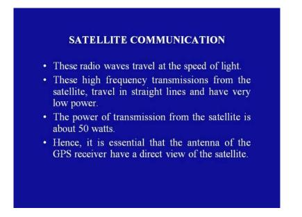
These high frequency transmissions from the satellite travel in straight lines and have very low power. It has been observed that the power of transmission from the satellite is about 50 watts. Hence, it is essential that the an10na of the GPS receiver have a direct view of the satellite itself.
