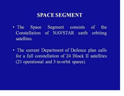
The next element is the space segment. The space segment consists of the constellation of NAVSTAR earth orbiting satellites. The currently, the department of defense plan calls for full constellation of 24 block II satellites, out of which 21 are operational and 3 are in standby mode. Out of this 21 satellites which are there, these satellite are placed in 6 orbital planes which are inclined 55 degrees to the equator.
