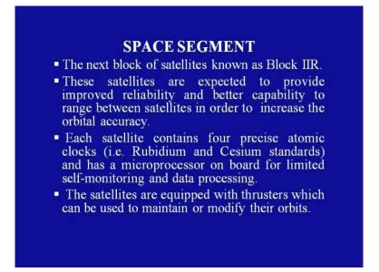
The next block of satellites known as block II R. These satellite are expected to provide improved reliability and better capability to the range between the satellites in order to increase the orbital accuracy. Each satellite consists of 4 precise atomic clocks that is rubidium and cesium standards and has a microprocessor on board for limited self monitoring and data processing. The satellites are also equipped with thrusters which can be used to maintain or modify their orbits.
