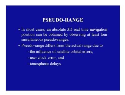
In most cases, an absolute 3 dimensional real time navigation position can be obtained by observing atleast 4 simultaneous pseudo ranges. These pseudo ranges differ from the actual range due to the influence of satellite orbital errors, user clock errors and ionospheric delays. With this knowledge regarding the GPS system, the user is now ready to take the observations. So, in the next session I shall discuss the various GPS positioning methods.
