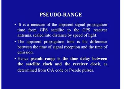
Now, coming to the pseudo range; it is a measure of the apparent signal propagation time from the GPS satellite to the GPS receiver antenna, scaled into distance by time by scaled into distance by speed of light. The apparent propagation time is the difference between the time of the signal reception and the time of emission. Hence, pseudo range is the time delay between the satellite clock and the receiver clock as determined from C/A code or P code pulses.
