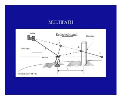
This particular slide it shows a line diagram as to how the multipath delay causes a difference in the times range of the signal being received at the GPS.
