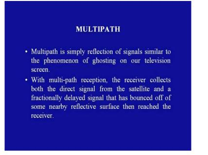
Then, multipath; multipath is simply reflection of the signals similar to the phenomena of ghosting on our television screens. With multipath reception, the receiver collects both the direct signals from the satellite and a fractionally delayed signal that has bounced off from some nearby reflective surface, then reaches the receiver.
