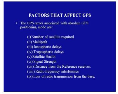
So, let us to look at what are the factors which affect GPS. The GPS errors associated with absolute GPS positioning modes are; 1.Number of satellites required, 2.Multipath, 3.Ionospheric delays, 4. Tropospheric delays, 5. Satellite data, 6.Signals strength, 7.Distance from the receiver, reference receiver, 8. Radio frequency interference and 9 is loss of radio transmission from the base.
