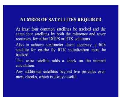
So, at least 4 common satellites be tracked and the same 4 satellites by both the reference and rover receivers either in DGPS or RTK solutions be there. Also, to achieve centimeter level accuracy, a fifth satellite on-the fly RTK initialization must be tracked. This extra satellite adds a check on the internal computations. Any additional satellite beyond 5 provides even more checks which is always useful.
