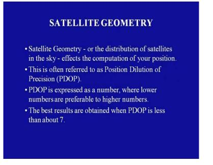
Then is satellite geometry; satellite geometry or the distribution of satellites in the sky effects the computation of your position. This is often referred to as position dilution of precision or in short, PDOP. PDOP is expressed as a number where lower numbers are preferable to higher numbers. The best results are obtained when PDOP is less than about 7.
