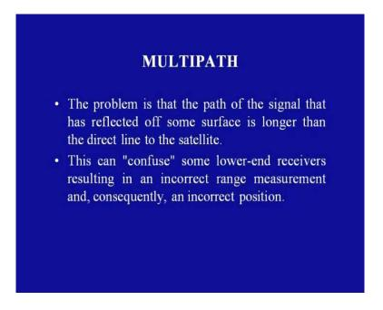
The problem is that the path of the signal that has reflected of some surface is longer than the direct line of the satellite. This can confuse some lower end receivers resulting in an incorrect range measurement and consequently an uncorrected position.
