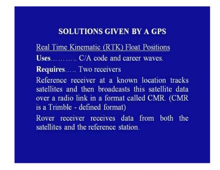
Next is real time kinematic; RTK float positions. Well, this solution requires C/A code along with carrier waves. It requires 2 receivers; the reference receiver at a known location tracks the satellites and then broadcasts this satellite data over a radio link in a format called CMR, CMR is Trimble - defined format. Rover receiver receives data both from the satellites and from the reference data.
