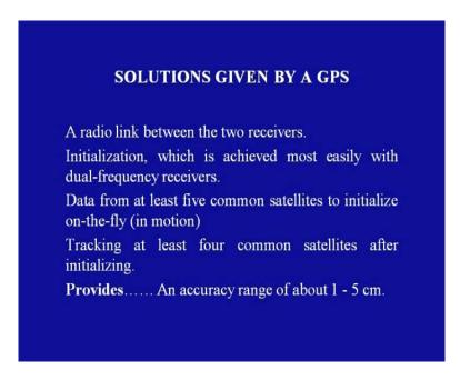
A radio link between the 2 receivers has to be maintained. Initialization, which is achieved most easily with dual - frequency receivers. Data from at least 5 common satellites to initialize on the fly that is in motion are required and one needs to track at least 4 common satellites after initialization procedure.
