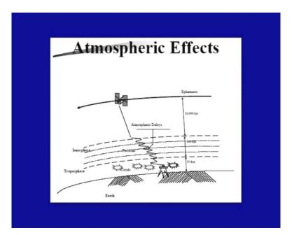
This particular slide, it shows the atmospheric effects on the signal, GPS signal which is received by the antenna. And, one can see there are two layers which cause this problem; ionosphere which is approximately 200 kilometers above the earth surface and troposphere which is the approximately 50 kilometers above the earth surface.
