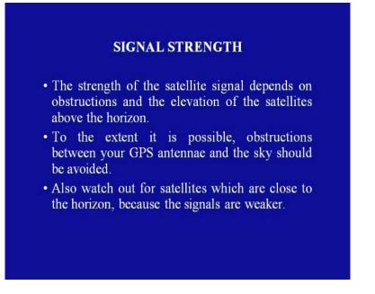
Then is signal strength. The strength of the satellite signal depends on the obstructions and the elevation of the satellites above the horizon. To the extent it is possible, obstructions between your GPS antennae and the sky should be avoided. Also, watch out for satellites which are close to the horizon because signals are weaker.
