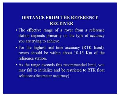
The next factor which may effect the GPS observations is the distance from the reference receiver. The effective range of a rover from a reference station depends primarily on the type of
