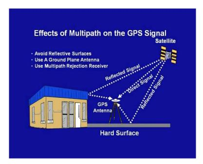
This particular slide shows the phenomena of multipath. We can see that the GPS antenna has been located on a hard surface and closed by there is building which has some reflective
