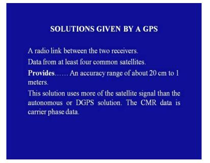
A radio link between the 2 receivers is required. Data from at least 4 common satellites need to be tracked both by the reference and the rover GPS receivers. This type of solution provides an accuracy range of about 20 centimeters to 1 meter. This solution uses more of the satellite signal than the autonomous or DGPS solution. The carrier data, this CMR data is a carrier phase data.
