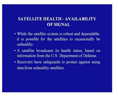
Ehen the satellite system is robust and dependable, it is possible that the satellites to occasionally be unhealthy. A satellite broadcasts its health status based on the information form the US department of defense. Receivers have safeguards to protect against using data from unhealthy satellites.
