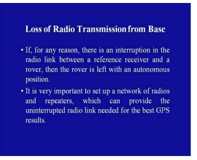
Then loss of radio transmission from base; if for any reason there is an interruption in the radio link between a reference receiver and a rover, then the rover is left with an enormous autonomous position. It is very important to set up a framework of radios and repeaters which can provide the uninterrupted radio link needed for the best GPS results.
