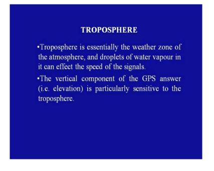
The next factor is troposphere. Troposphere is essentially the weather zone of the atmosphere and the droplets of water vapour in it can affect the speed of the signals. The vertical component of GPS answer that is elevation is particularly sensitive to the troposphere.
