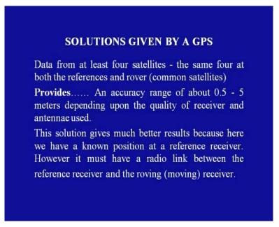
Data from at least 4 satellites; that is the same 4 at both the reference and rover receivers are required. It provides an accuracy range of about 0.5 to 5 meters depending upon the quality of the receiver and the antennae used. This solution gives much better results because here we have a known position at a reference receiver. However, it must have a radio link between the reference receiver and the rover; that is the moving receiver.
