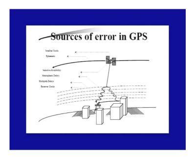
Before we proceed ahead, this particular slide shows a schematic diagram of the sources, radio sources of errors in GPS observations. First error which could be which needs be looked into is through cost by the number of satellites. As we know that apart from the spatial coordinate's x, y and z, time is another factor to be taken into consideration.
