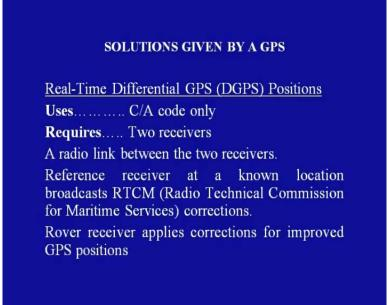
The next solution is real time differential GPS or DGPS position. Well, this type of solution uses a C/A code only and requires 2 receivers. Between the 2 receivers, a radio link is required. The reference receiver at a known location broadcast RTCM that is radio technical commission for maritime services corrections. The rover receiver applies corrections for improved GPS positions.
