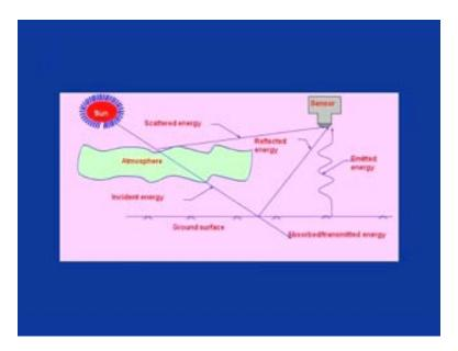
This slide shows a schematic representation of the electromagnetic radiation interacting with the atmosphere and thereafter on reaching to the earth surface, the interaction that takes place. Based on the interactions which take place, the energy reflected both from the atmosphere and from the earth surface is now recorded by the sensor.
