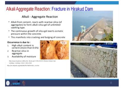
Then this type of hydrolysis is also sometimes plays very dangerous to the engineering structures. For example here alkali-aggregate reaction and fracture in Hirakund Dam. So that is why how what is this alkali-aggregate reaction? If you want to understand it if you see here
