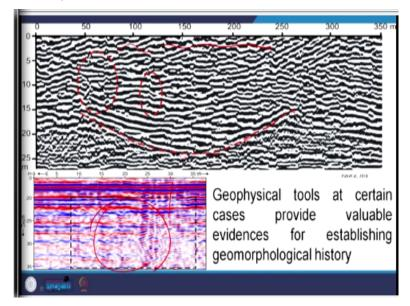
For example if you see here, these 2 are the ground penetrating radar profile. In ground penetrating radar profile, if you see here the red mark, it is a paleochannel surfacial sediments that burying it. If we do not have this geophysical profile or this radar profile, we cannot say whether in the past a fluvial system was active here, is not it. So that means some cases similarly here this is a paleochannel buried under sediment.
