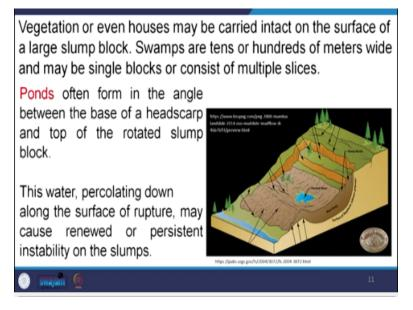
Vegetation or even houses may be carried intact with the surface of failure, the large slump block. Swamps are 10's of 1000's of meter wide and may be single block or consist of multiple slides sometimes, ponds are generated here. For example, if you see in this figure, here these different blocks; this is one block, this is another block; the blocks are detached gradually and are moving rotational motion.
