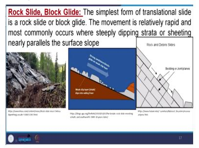
So, in this figure if you see, these are this rock slides and here the rock sliding is there, this is the block glide, the block glides are there, so along this plane these rock material is going down. (Refer Slide Time: 22:32)
