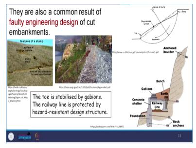
For example, here the faulty engineering structure, suppose here we are removing the material, so that means we are creating a cliff which can free fall here, which can slump down, so in that case, what we generally do; here, we are creating the gabions, the walls composed of boulders, it is tied with nets, with metal nets, if you see here is a metal or plastics or some types of polymer is there, these nets, so that means, we are allowing the water to percolate, water is removed.
