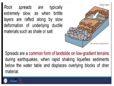
Rock spreads are typically, extremely slow as when brittle layers are rafted along by slow deformation of underlying ductile layers or ductile materials. Spreads are common form of land slide in low gradient slopes, low gradient terrains, during earthquake, when rapid shaking liquefies the sediment below, the water table and displaces overlying rocks in the drier material, so if we have this liquefaction occurs below the water table, the whole material try to move off.
