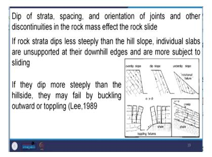
Dip of strata, spacing and orientation of joints and other discontinuities in the rock mass that effect the rock slide, if rock strata dips less than that of the hill slope, so individual slabs are unsupported at the downhill edges and are more subjects to slides. If the dip is more than the or the dip is more, it is steeply dipping than the hill slide, it may fail and looking outward the toppling.
