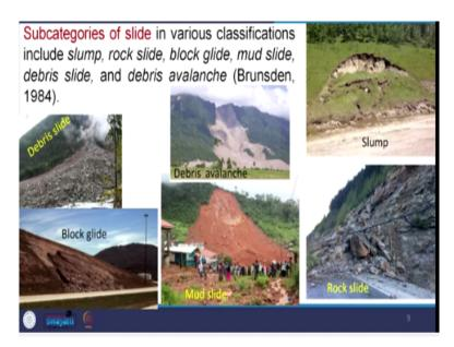
Subcategories of the slide in various classifications are there that is include, slump, rockslide, block glide, mud slide, debris slide and debris avalanches, so here some figures are given, this figure denote to slum; slumping of material here, then debris avalanches; avalanches very rapid movement, avalanches, then debris slide, it is sliding down, then rock glide, this rock; intact rock, if you see here this whole rock as a whole block, it is gliding down, it is block glide.
