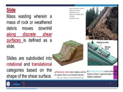
Then, another type of mass wasting, it is called slide, where a mass of rock or weathered debris moves downhill along the discrete shear surface that is a plane, a definite plane is associated, on a definite plane, if rock mass may slide, debris may slide, anything may slide on this surface, so this defined surface is there. So, based on the defined surface that is why it is called slide, it is sliding down.
