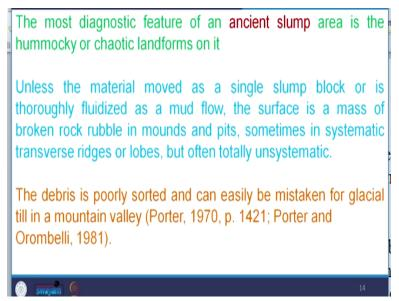
The most diagnostic features of an ancient slump area is the hummocky or chaotic landforms on it, it is very important here, this diagnostic characteristic of ancient slumps, ancient slump has to be understood properly to go for in proper engineering design otherwise, suppose for example, in an area, we are assigned for engineering development or road alignment or so, we do not recognise the ancient slumps.
