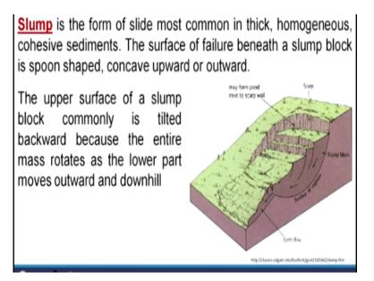
If you see in this figure, this is the plane of failure, it is concave upward, it is like a spoon shaped, so once the material is sliding from here, detached from here, it has to undergo a rotational motion and here it is concave upward and this side if you see here, this is convex upward, so the upper surface of a slump block is commonly is tilted backward because the entire mass rotates at the lower part moves upward in the downhill.
