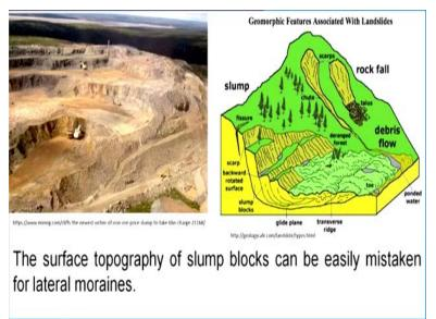
Here the surface topography of slump blocks can be easily mistaken with lateral moraines, for example, if you see here, these are this debris material is mined here and this is nothing, it is the slump material ancient slump material but it should not be mistaken for ancient moraines, okay
