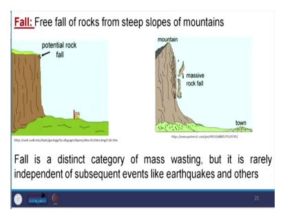
Then, another type of mass wasting, it is called fall, it is free fall, that means, only the air resistance will be there, so to prerequisite this for the fall, this, there should be a steep slope and there should be weathered rock material, there should be jointed rock material, so that this material which is detaching from this rock body, it is freely falling on the surface; freely falling to this valley and air resistance is the only resistance nothing else.
