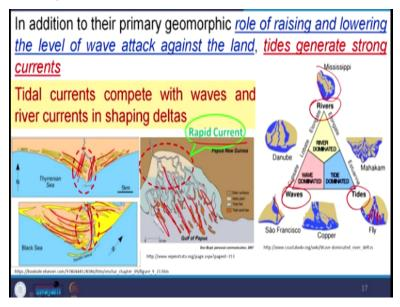
In addition to their primary geomorphic role of raising and lowering this level of wave attack against the land, tides generate strong currents; tidal currents compete with waves and river currents to shaping the delta. Here, not only this tides act as a lift of; lifting this water level or the wave level from here to here because in the low tide level, wave is acting at this level, at high tide level, wave is acting at that level.
