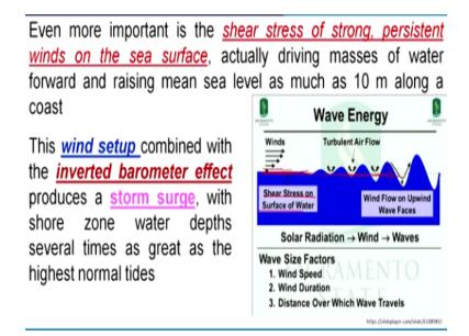
Even more important is the shear stress of strong persistent wind on the sea surface actually, driving mass of water forward and raising mean sea level by 10 meters along this coast. So, during the cyclone and due to this shearing action of these high speed winds, so if you see here, this is the water surface or ocean surface and wind is blowing here, this is the shear stress on the surface of water.
