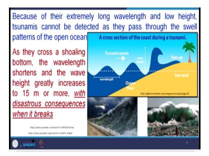
And finally, these are changing the geomorphic process along this coastal region because of their extremely long wavelength and low heights, tsunamis cannot be detected as they passed through the swell pattern of the ocean flow, as they cross the swelling bottom, the wavelengths shortens and the wave height greatly increases up to 15 meter or more with disastrous consequence when it breaks.
