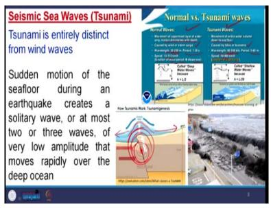
Then another reason or another way of generation of wave, it is the Tsunami waves, so Tsunami it is related to submarine earthquakes. So, if you see here this is a diagrammatic representation if you are creating an earthquake here, from the earthquakes, waves are moving upward and finally, it is swelling of this ocean water here and the wave it migrates this direction and this direction and hits the continental region.
