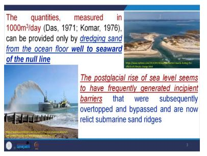
So, this quantity has to be measured and can be provided only by dredging out of sand from the ocean floor well seaward to the null line why because we know in last class. We are we can remember that the null line or the null point in a profile or null line along these coast parallel to the coast, this is a imaginary line which defines either sands to move seaward or is to move coastward. So, that null line and we know along this null line.
