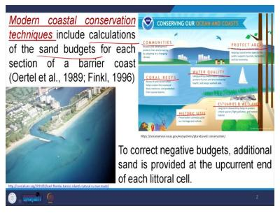
So the modern coastal conservation techniques that include calculations of the sand budget for each section of the barrier coast. So this is important calculation of this sand budgets so that means suppose we have a sand sheet in a particular coast, so how much sand is there, how much sand is in mobile condition, which is in the permanent condition of below the sea level that is it matters to us. It matters to us how much sand is mobile, that means how much sand is renewing there.
