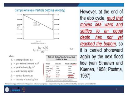
Now here is some of this analysis by Camp, it is settling velocity analysis it will say here we have different size classes, gravel coarse and fine sand, silt and clay and colloids. And if you see here this colloids and these clay to settle down up to 1 feet so 1 feet depth to settle down clay, it takes 10 weeks and this colloids it took 20 years for 1 feet of settlement. So, now imagine for every 6 hours we have tidal reversal, high tide and low tide.
