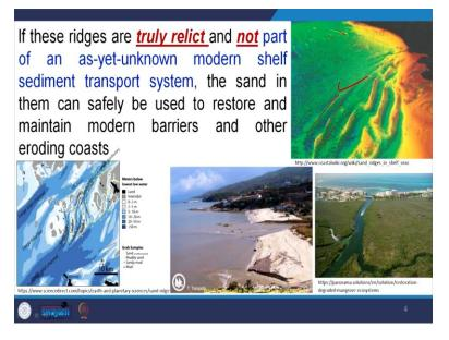
If these ridges are truly relict and not part of an as-yet-unkwon modern shelf sediment transport system, the sand in then can safely be used to restore and mainly modern barriers and other eroding costs. This is important to understand for this coastal management system, because we have sand ridges, which were formed during this postglacial rise of the sea level and there relict one for example.
