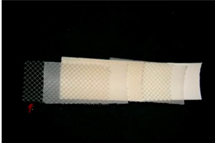
The layers of a spiral wound membrane
