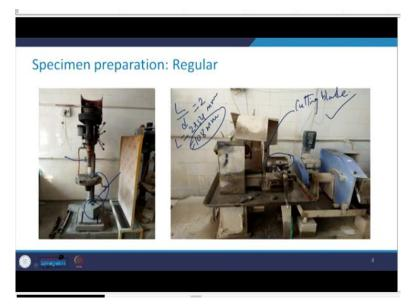
See here, these are the 2 pictures of the machinery that we have in our lab here at IIT Roorkee. So, if you just have a look here, see this is what is the small block that has been cut from a large block of the rock and then this is placed here at this platform. And then here you see that this is the drill bit. So, with the help of the motor which is mounted here, the whole assembly is brought down.
