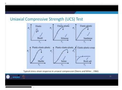
Some of the typically stress strain response in uniaxial compression. So, you see that for different type of rocks I have shown some figure. So, for basalt, it is elastic behavior. So, you see till peak it is going longer linear path and then suddenly it breaks. So, that is how it is. Now, in case of the siltstone the behaviour is elastic plastic, that means in the beginning it is elastic and then here this becomes plastic.
