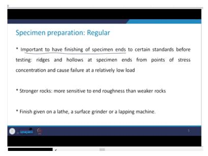
So, we need to be careful about that. So, it is very important for us to have the finishing of the specimen ends. Let us say this is the specimen. So, what I mean to say by a specimen ends are this end and this end. So, there should not be ridges or hollows here at the specimen ends. Because what will happen here is if you have these ridges and hollows when you apply the load, there is going to be the stress concentration at those points.
