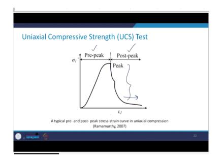
So, this is typically showing the pre peak and the post peak stress strain curve in the uniaxial compression. You can see that in the beginning till it reaches to this peak value with the increase in the stress increment or when you increase the stress in increment, there is the increase in the strain. Once it reaches the peak value, then beyond that, you see the stress levels are reducing.
