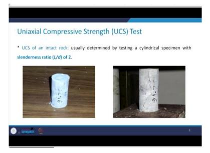
Now, these are the 2 pictures which we have taken after the conduct of the UCS. So, this was just to show you that how the specimen looks like, before I have already shown you and after the tests. This is the MTS machine; this has been taken from a textbook.
