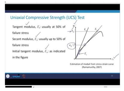
Another important aspect which we get from the UCS test, this information, which is the determination of the modulus. Now, there are different types of modules which have been defined, which are used in the design and the analysis. So, those have been explained here in this figure. So, you see that this figure is the plot between the axial stress and the axial strain. So, as we saw in the previous slide, the typical shape of this stress versus strain response is like this portion.
