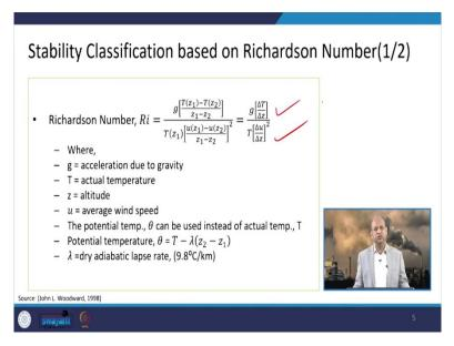
When we consider the Richardson number, this is defined as with this equation, we are you can see these are the parameters this g acceleration due to gravity, then  $T(z_1)$ ,  $T(z_2)$  at different heights temperature, and actual temperature at  $z_1$  and  $z_2$  height,  $z_1$  minus  $z_2$  means difference between the height or the elevation, and this formula is used to calculate this particular relationship and this gives the  $R_i$  your Richardson number.
