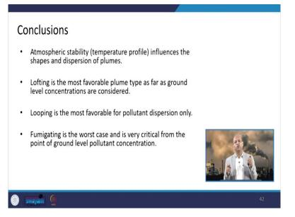
So, in conclusion, we can say that the atmospheric stability that is the temperature profile, this influences the shapes and the dispersion behaviour of the plumes. And the lofting is the most favourable plume tie for us because we always want that the pollutant concentrations should not build up on the ground level, the concentrations should not be high at the ground level it goes and dilutes in the atmosphere, that is fine for us.
