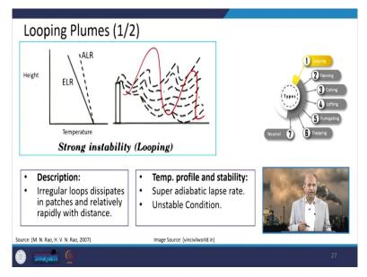
Looping plumes means the plume when it comes out then it goes up and down and dispersion happens very quickly and the reason is because the ELR that is the Environmental Lapse Rate actual lapse rate is higher than the adiabatic lapse rate. So, the atmosphere is unstable and turbulence is low and depending upon this turbulence this fluctuation will go like it will go up it will come down.
