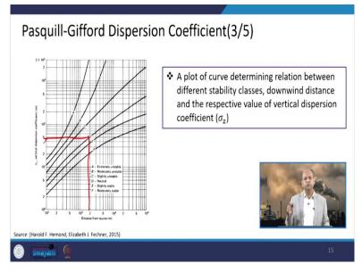
Similarly, sigma z So, these are the plots which show the variation of vertical dispersion coefficient and the distance from the source horizontal distance. So, again if you take the 2 kilometre or 2000 metre and go up to D, then you can get this value of sigma z. So, that is the very simple way of getting sigma y and sigma z which will be used for estimating concentrations in Gaussian dispersion models.
