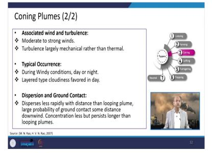
And you can see like, moderate or strong winds are the kind of properties which signify these particular phenomena, turbulence largely mechanical rather than thermal, and this during windy conditions, day or night it can occur and layer type cloudiness can be there which can favoured in the daytime.
