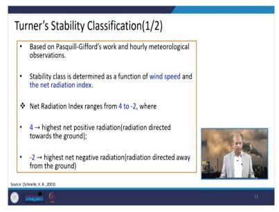
Well, the Turner's stability classification with which you can determine upon the basis of Pasquill-Gifford work and hourly meteorological observations and the stability class is determine as a this function of wind speed and the net radiation index. A net radiation index may range from 4 to minus 2 where, 4 is highest net positive radiation, radiation directed towards the ground and minus 2 highest net negative radiation, radiation directed away from the ground.
