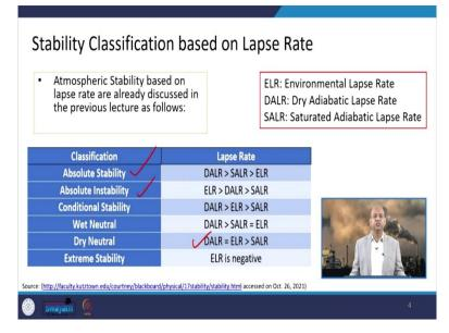
So, when this ELR is less than both DALR and SALR or you can say DALR is greater than SALR, which is always there and SALR is also greater than ELR in that case, the atmosphere is absolutely stable basically, when this environmental lapse rate is greater than DALR means the actual temperature gradient is faster, means temperature is decreasing faster than the theoretical lapse rate of the DALR, then this is absolutely unstable or instable.
