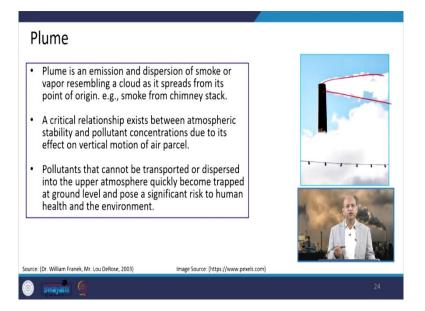
Well, when we talk about the plumes, the plume is nothing but, the emission of the these exhaust gases or particles and the dispersion of the smoke or vapour you can see and resembling as a cloud it goes down and spreads from a point of its origin. So, from like stack or wherever, something happens like this and it disperses according to the wind velocity according to the stability classification.
