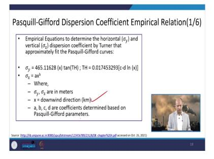
Like, this is one empirical relationship  $\sigma_y = 465.11628$  (x) tan(TH); TH = 0.017453293[c-d ln (x)] and theta (TH) is given by this relationship where C D and A and B are some sort of coefficients, sigma y, sigma z are a metres, downwind distances are in kilometres. Whereas, in graph it was in metres distance was in metres please remember. A, B, C, D are coefficient determined based on Pasquill-Gifford parameters.
