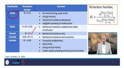
So, according to the Richardson number we can again define the stability classification of that atmosphere for example, if  $R_i$  is greater than 0.25, then it is the atmosphere is stable and in stable atmosphere no vertical mixing. Weak winds and then strong inversion may also happen. Mechanical turbulence is dampened, negligible spreading of smoke plume is there in a stable atmosphere.
