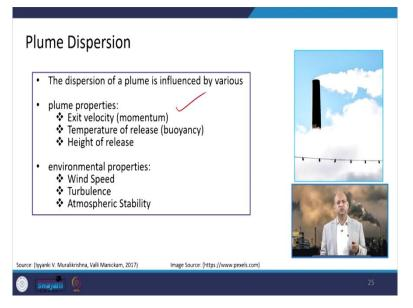
Well, so we can see the plume dispersion depending upon it is, influenced by several properties like exit velocity, stack velocity or there are plume properties you can call. Exit velocity from the stack, temperature of the release that buoyancy, exit velocities momentum, height of the release even diameter all those things are there.
