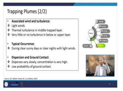
And this happens like light wind thermal turbulence or dispersion very slowly concentration is very high in that particular layer and low probability to come in contact with the ground because, this is as I said trapped and it can, move in the horizontal direction with the horizontal windward vertical distribution is restricted.
