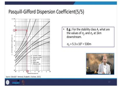
Well, for an example, like for if you are given the stability class A like I just show for stability class D, but if it is a stability class A and the values of sigma y and sigma z are determined at 1 kilometre, then 1 kilometre is nothing but 1000 metre. So, here you go up to this A, this is the A and you go this side, so, you get this value.
