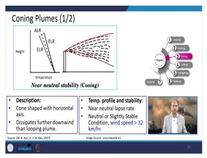
When we talk about coning it happens when like near neutral phenomena means, the actual environmental lapse rate is almost near to the ALR. It may be parallel or just a little bit, higher side lower side does not much matter. And this cone means, vertical movement can happen on both sides upper and lower and like a funnel or cone, the dispersion happens that is why it is known as coning.
