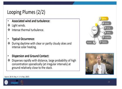
And you can see the associated wind and turbulence properties like light wind maybe there, then thermal turbulence are intense. And the occurrence may happen like daytime with clear or partly cloudy skies, intense solar heating must be there. So, that gradient of temperature is faster than or more than this ALR Adiabatic Lapse Rate.
