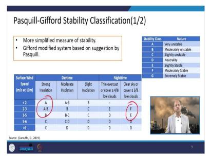
Well, when we talk about Pasquill-Gifford stability classification, then they give very good relationship between the surface wind velocity, surface wind velocity means the velocity which we have measured at the 10 metre height from the ground, that we call the surface wind velocity. Then the strong insulation or moderate insulation or slight insulation that is in the daytime. In night-time, they have two categories depending upon the cloud cover.
