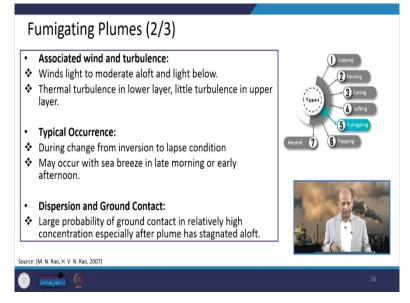
And these are the conditions when it occurs like during change from the inversion to the lapse conditions, it may occur also with the Seabreeze in the late morning or early afternoon, when upper layer maybe their inversion remains and the lower inversion breaks. So, a lot of turbulence and instability is there at the lower layer and the dispersion may happen very quickly.
