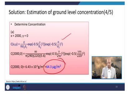
And when we go away from the centerline, 0.1 kilometer, 100 meter away from the centerline, then the estimated concentration is 60.6. So, you can see, it was 64 and now it is 60. That means the concentration is decreasing when we go away from the central line. So, very simple to understand that particular concept, that as we go away from the centerline concentration decreases.
