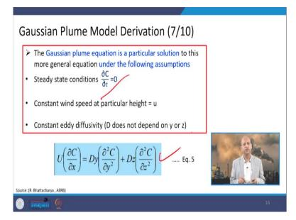
Now, you see further you can have this steady state condition that means with respect to the time concentration is not changing, change rate is zero. So, this when we put then that particular equation give this kind of relationship.
