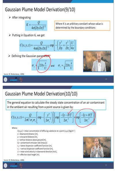
Ultimately, we get this relationship where  $\sigma y$  is this terminology. So, the final equation of the Gaussian dispersion model is in this form, where Q is this emission rate divided by  $2\pi$  into U. U is the average wind velocity at the stack height, effective stack height.  $\sigma y$ ,  $\sigma z$ , those components which are related to diffusivity coefficient X Y U is terminology is there. So,  $\sigma y$  and  $\sigma z$ , they also incorporate these values x.
