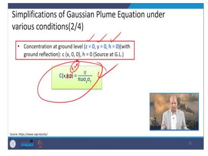
Similarly, if we go for like even stack height is 0 means like some heap of the leaves is built. So, how this person will occur? What would be the concentration at certain distance? So, in that case Z = 0, Y = 0 and H = 0. Stack is not there. At the ground level only something you are burning and emission is occurring. So, in that case, this becomes very simple. So, C (x, 0, 0) and H = 0. In that case this kind of relationship we use.
