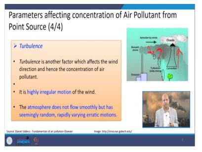
Then the turbulence. Turbulence is the parameter like normal direction is there in which wind is flowing. But turbulence is within that wind, pockets of the wind, they have different direction, away or other than the main direction, like these the eddies, it goes up, it comes down, a lot of turbulence occurs in the fluid motion, whether it is here or water something like that.
