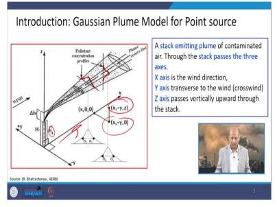
So, this is very important figure for introducing this Gaussian plume model from the point source. So, here point source is the stack. You can see this stack is having stack height  $h_s$ , small  $h_s$ . This H is the effective stack height. Because  $h_s$  is added with the  $\Delta h$ .  $\Delta h$  is the plume rise and plume rise happens, as I repeated earlier also that because of buoyancy.
