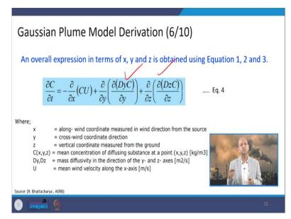
Then we do the summation of those. So, the concentration that overall expression of the concentration variation with respect to the time  $\delta C$  by  $\delta t$  is like  $\delta$  by  $\delta X$  into C U minus terminology plus these dy and dz, these are the mass diffusivity coefficients, which are in the Y direction and Z direction, they are taken into account along with this concentration. So, the summation of these three components give us the concentration with respect to time.
