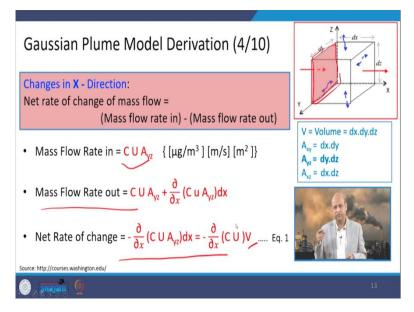
Now, if you see like mass flow rate, so, mass flow rate is nothing but concentration multiplied by the u that wind velocity and then the area. So, area into wind velocity u, that will give certain value and then if we multiply with dx that distance, so, this area into the short distance will be the volume.
