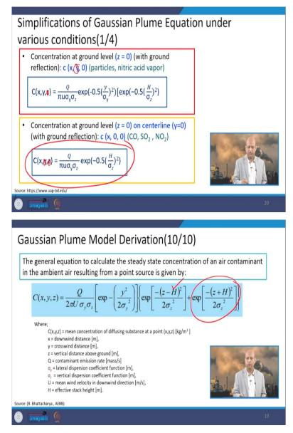
Now, there are some special cases, for example, we want to calculate concentration at the ground level. So, ground level means Z = 0, height coordinate is not there, Z = 0. And with
