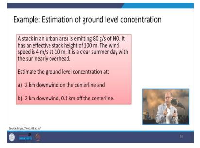
Now, if you want to give some example, how to estimate the ground level concentration. So, this is one very small example you can try like a stack in an urban area is emitting 80 gram per second of nitric oxide. It has an effective stack height of 100 meter. So, the effective stack height is given.
