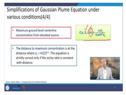
For that, we go for these kind of relationships, there are some empirical relationships which have been derived, this is X component is there, effective stack height and at the ground level at the centerline, so, Y = 0 and Z = 0. This is the relationship you can have. The maximum ground level concentration from elevated source is given by this formula.
