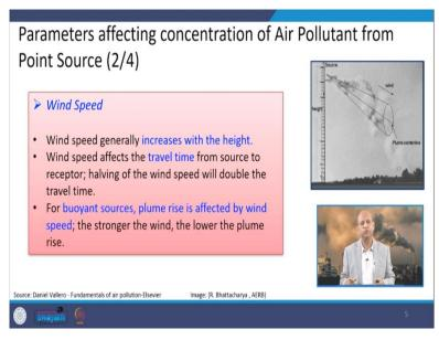
Now, if we see this wind speed, so, it has like it affects the travel time from source to the receptor and having the wind speed like half of the wind speed, then it can double the travel
