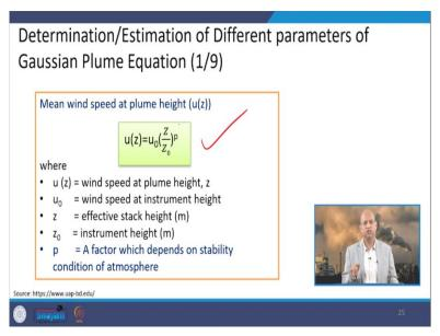
They will influence, basically, this wind velocity, because when we want to calculate wind at different heights, we use this particular formula, where p is this constant value effector with dependence upon the stability conditions of the atmosphere. So, u = 0 is at the Z = 0 height and u (Z) is at the Z height and this component (Z/Z<sub>0</sub>) power of p. So, this equation has to be used. And where this p is derived?
