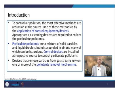
And one of these methods which are prominent or effective to control the air pollution emissions is by the application of control equipment or devices at the source itself. And appropriate air cleaning devices are required to collect the particulate pollutants, because whenever there are a number of pollutants are emitted. So, as per the nature of the pollutant, whether it is particulate pollutant or gaseous pollutant we have to install some equipment or controlling devices.
