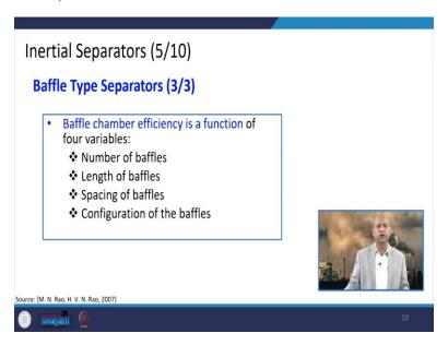
And these baffle chamber efficiency is a function of four variables basically, like number of papers we have provided, length of the baffle, spacing of the baffle, configuration of the baffles, the types etc. So, these things will influence the separation of the particles basically.
