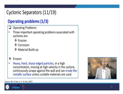
Well, operating problems are there, like it can eroded by particulate matter because it strikes to the surfaces, corrosion maybe there if those gas, carrier gas is having like acidic content like SO<sub>2</sub> etc. then material build-up can be there at the inlet, outlet or some surfaces also. So, at some surfaces sometimes people use those kind of like rim kind of thing and it can be removed, otherwise regular cleaning is needed.
