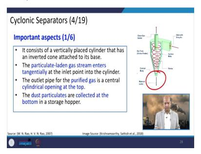
Important aspects like it consists of vertically placed cylindrical apparatus that has an inverted cone kind of attached to the base. And the particulate laden gas stream enters tangentially, at the inlet point here and then it goes down. And the dust particles are collected at the bottom in the storage hopper.
