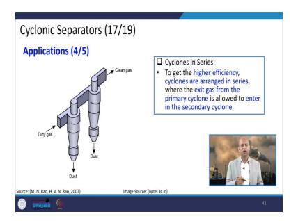
If we go into series only one after one then dirty gas goes to one particular this separator then cleaner gas goes to another separator that way you can ensure very high efficiency or very clean gas at the outlet depending upon how many cyclone separators you have installed in series basically.
