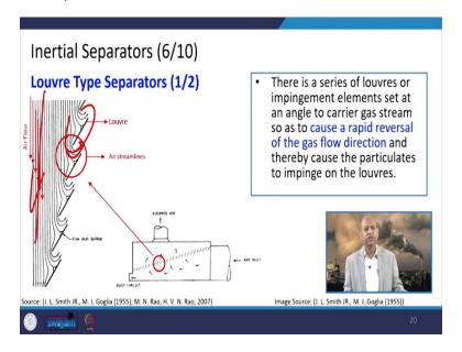
You can see like this louver type of separators where these kind of louvers are installed. So, that there is the change of the velocity, like air is going like this, but nearer to these kind of insertions this air changes its velocity and then this it causes rapid reversal of the gas flow direction and thereby it causes the particulate matter to impinge on the louvers and lose the velocity and get
