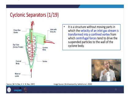
Now, we come to the cyclonic separators. So, in cyclonic separators basically it is nothing but a structure without moving parts in which the velocity of an inlet gas stream is transformed into a confined vortex that circular motion from which centrifugal forces tend to drive the suspended particles to the wall of the cyclone body. So, like for example, this inlet is there and this gas goes downwards basically, it goes downwards in circular motion.
