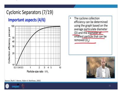
In this graph the efficiency, collection efficiency depending upon the size of the ratio of the particle, this D and D, particulate diameter D and diameter of smallest particle that can be removed D<sub>p</sub>. So, if it is like 10 up to 100 it can be removed. So, the ratio and you can decide the efficiency.
