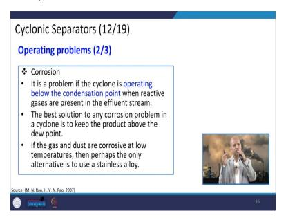
And corrosion-related means the carrier gas is taken into at the temperature where dew point is not achieved only then it would be better, otherwise corrosion problem may be there.
