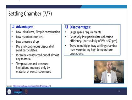
Then there are advantages and disadvantages. In advantages that it is low initial cost, simple construction. The construction is very simple kind of chamber you can divide. But in terms of disadvantage it requires large space. So, in countryside it can be okay fine, but in urban areas it is difficult because land cost is much more.
