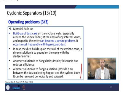
And metal build-up can be taken into consideration and it can be removed by this rim provision or by regular cleaning.
