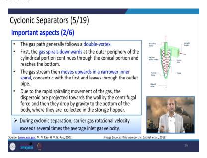
The gas path generally follows a double vortex. Once it comes down then it goes up inside. So, double part is there. So, that way there is a possibility of collection of smaller particles also. During
