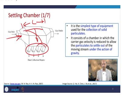
So, if we start our discussion on settling chamber that is the simplest device. Basically, this is simple chamber, length, width, height, so this kind of device. So, there is inlet, gas, lead and by
