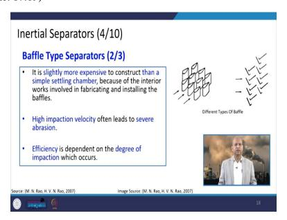
Whenever this high impaction velocity often leads to severe abrasion, so those are the issues basically. Efficiency is dependent on degree of impaction which occurs. So, those things we have to ensure if we want to remove more particles.
