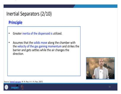
So, the principle, basically the inertia related, inertia when you change the direction by baffles etc. inertia occurs and they strike to the surface then they lose the velocity and slide down. And we, these solid moves along the chamber with the velocity of the gas gaining momentum and it strikes at the barrier and get settles down when air changes the direction because of losing the velocity.
