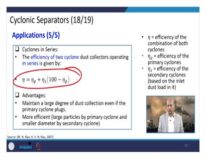
So, if you want to calculate the efficiency in cyclones installed in series, then this is the simple formula like eta equals eta p plus this eta s 100 minus np [  $\eta = \eta_p + \eta_s (100 - \eta_p)$ ]. So, this is basically this eta ( $\eta$ ) efficiency of the combination of
