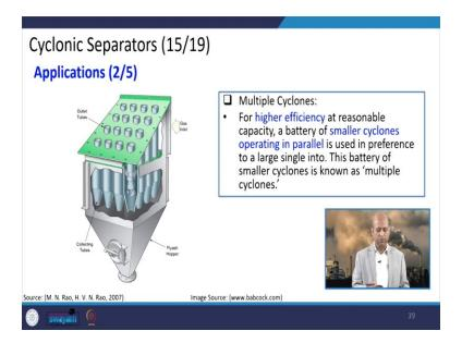
For example, to increase the efficiency in row and parallel rows as well as this kind of system maybe there where smaller cyclones can be put together and multiple cyclones we can call it so that more cyclones are available to remove the particles.
