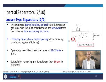
And it is suitable for removing particles larger than 30 micrometer. So, that way again it is better than the settling chambers, but baffle walls are better than these.
