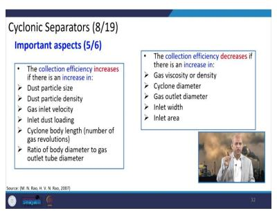
Well, the important aspects like the collection efficiency increases, if there is an increase in like dust particle size or dust particle density or gas inlet velocity or inlet dust loading or cyclone body length, number of gas revolutions because it will ensure more gas revolutions, then ratio of the body diameter to the gas outlet tube diameter. And the collection efficiency decreases with the gas
