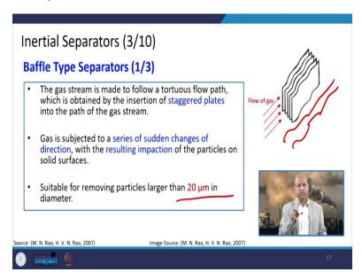
When we talk about baffle type separators, these kind of deformed kind of valves we take so the direction changes continuously and the suitable for removing particles larger than 20 micrometer in diameter. So, that way it is better if we compare with the settling chamber. So, certain change direction is to be ensured by these staggering kind of plates etc.
