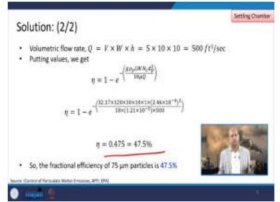
So, we put all these values and we calculate this efficiency and it comes around 47.5 percent. So, you can say that the fractional efficiency of 75 micrometre particles is around 47.5 percent or 48 percent. So, that much it is removed others may just bypass you can say like that short circuit kind of thing.
