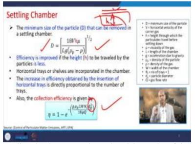
So, as we go for settling chambers as you know the minimum size of the particle diameter which can be removed in a settling chamber is given by this particular relationship where D is the diameter of the particle and then there are other parameters like horizontal velocity of the carrier gas which contains the particulate matter.
