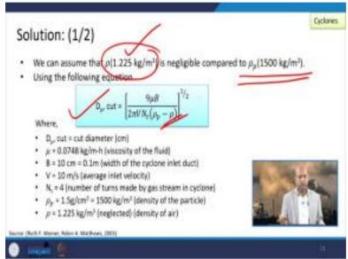
So, we use these values in this particular relationship, diameter cut, we calculate, we put these values of the density which is air density is negligible in comparison to the density of the particle which is 1500 kilogram per cubic meter. So, you can put here and you can ignore this parameter basically and all other values are given here.
