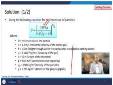
So, we use this particular relationship to estimate or to calculate the minimum size of the particle which can be removed fully. So, this is the relationship, we have all these values, v, h, mu, Lg, rho  $p(\rho_p)$  rho  $(\rho)$  all these values are there. So, we can put these values in this particular relationship and calculate the diameter.
