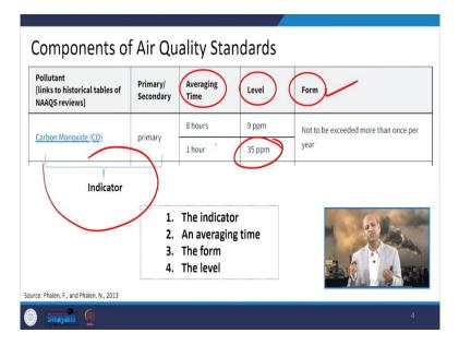
Well, when we talk about the components of air quality standards, so there are basically four basic components like the indicator, indicator means some pollutant like  $SO_2$ ,  $NO_2$  or carbon monoxide, whatever pollutant we are talking about that is the indicator and we also know whether it is primary pollutant or secondary pollutant.
