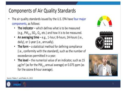
So, these pollutants are the indicators which are defined in terms of measurements which can be measured properly and the averaging time can vary from 1 hour to 8 hour 24 hour and annually also or monthly also the form is basically statistical method defining their accidents.
