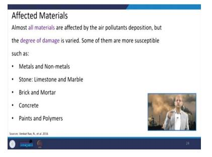
So, when we talk about how materials are affected, so we can see all kinds of materials are affected by these air pollutants, whether they are metals or non-metals. Even stones like limestones or marble, and then brick, and mortar, concrete, paints and polymers; all these building materials are damaged in one or other way by air pollutants. And we will see how they are damaged.
