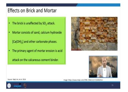
When we talk about brick and mortar, the mortar again has certain calcium carbonate related things. So that is affected, but brick is not so much affected by  $SO_2$  attack. So, you can see the mortar only, those gaps are because of this acid rain you can see.
