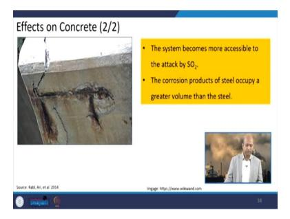
When we talk about the concrete, so in concrete basically this reinforced concrete. Basically, this is about the reinforced concrete. So, like these steel rods, iron rods are there. So, they are damaged by acid rain; and rust happens and then volume increases. So, further cracks developed in concrete and then concrete damage also happens. When we talk about this, this kind of gaps; so you can see this corrosion starts and then damage continues.
