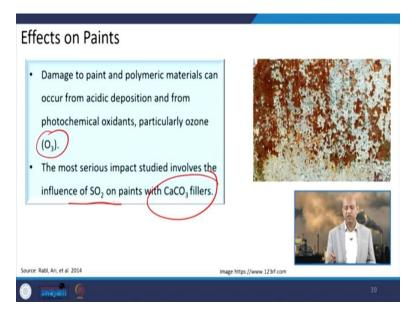
And on paints also, there are paints which can be damaged by like Ozone; because it is very oxidizing highly oxidizing gas as you know. So, because of these, then there is presence of certain calcium carbonate fillers in the paint; so, that can get affected by SO<sub>2</sub> also. But, ozone
