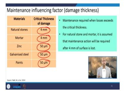
When we want to analyze the maintenance influencing factors like damage thickness etc; so you can see like natural stone 4 mm is there; these are the critical thickness basically. Mortar 4 mm, zinc 50 micro meter only; galvanized steel 50 micro meter, paints 50 micro meter. This much of thickness damage is there, then it is critical. And one should go for some remedial measure; otherwise, it will be highly damaged after some time.
