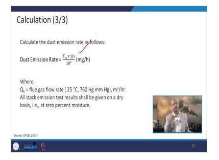
Then if you want to calculate the dust emission rate then we have to multiply it with the flow rate Qs, so that can give the emission rate.
