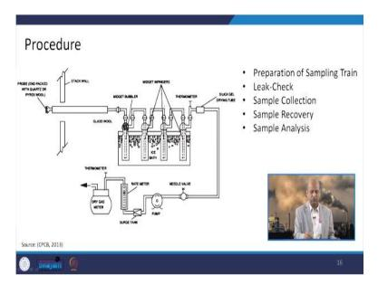
Then the procedure is shown in this particular figure, a schematic diagram you can see here, so the sample is collected and then sample is recovered and then it is analyzed in the laboratory. So, here you collect the sample it goes through these impingers and it is absorbed and then it is taken to the lab.
