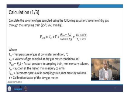
Well, so when we calculate the volume of the gas which has been sampled basically, so we need this particular relationship where pressure difference is there, volume of the gas sample at dry gas meter conditions and the temperature etc, so that correction can be applied according to their unit and then this gives the value of gas sample basically.
