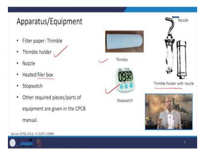
So, you can see there are other parts like filter paper or thimble which is known, then the thimble holder, nozzle is also there, then heated filler box, stopwatch is there and other parts of this equipment which are shown in CPCB manual basically you can go through that to learn more.
