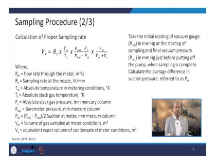
So, this is the calculation procedure for sampling rate basically where there are different parameters like flow rate, then the sampling rate, absolute gas temperature, absolute temperature of the metering conditions, then barometer pressure all these parameters are noted and we use those parameters here in this particular equation to calculate the sampling rate.
