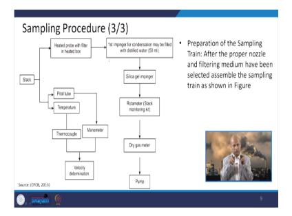
And if we talk about the sampling procedure basically so the two streams are there, one is like giving the temperature related, velocity related values, other one is giving us where this particulate matter will be collected, so the two streams you can look into in this procedure.
