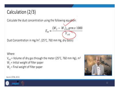
This value is used for like to divide this weight difference and it will give the concentration, concentration means weight divided by the volume flow rate, so this equation can be used for that purpose.
