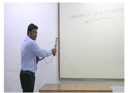
So, this probe is attached with this tablet. So, in this tablet a software has been installed in this tablet from which we are able to monitor the indoor air pollutants at various locations. So, what we need to do, we simply need to just attach this probe in this particular tablet and at any locations.
