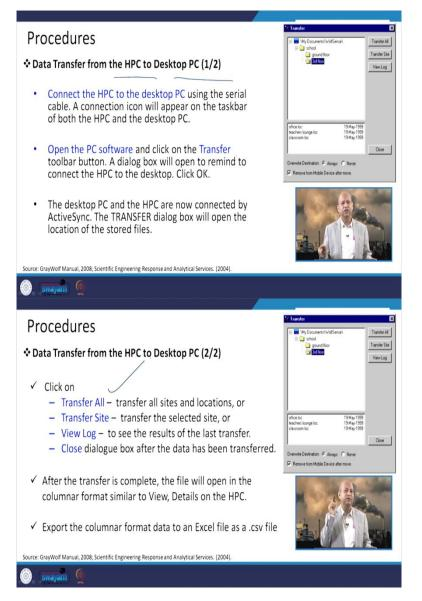
So, the data transfer takes place when we connect it with the desktop PC, and then this popup menu is there to transfer the data and the data is transferred then it can be opened in Excel sheet or different kind of software basically. So, you can see these are the possibilities transfer all if we transfer all the data which are stored there or transfers site specific data. So, those kinds of facilities are there.
