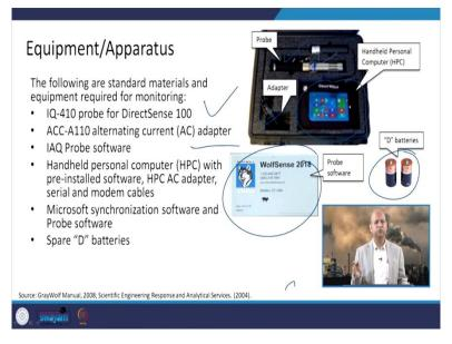
Well when we talk about the equipment means different parts or components of the instrument then we can see here one is probe and then this is handheld personal computer HPC and adapter is there so that you can directly use with AC otherwise batteries we can use for running this probe based monitoring. So, this is the sensor based monitoring equipments and this is IQ 410 probe which is used for the direct sense of hundred. It is known as per their parameters handling.
