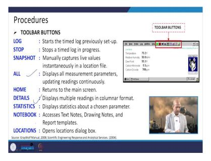
Toolbar button says like log, stop, snapshot, all these buttons so, this log is to start the time log previously which has been stored and then Stop button is to stop the that functioning or the reading, snapshot can be taken manually and all button gives all measurement data related to parameters which can be seen. So all these statistics, notebook, locations, they have their own functioning which we can look into.
