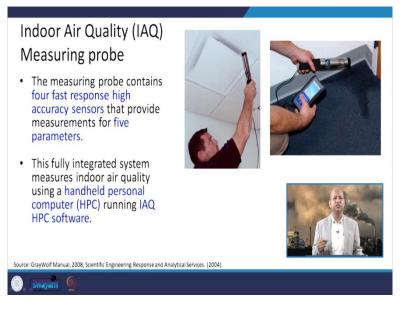
So, if we talk about how to use this probe or sensor based equipment, so anywhere indoor environment, you can take this probe and keep there for certain time. So, it has certain reactions and then it can give the reading of those particular components whether it is gasconcentration or humidity or temperature etc plus it can record the data into this HPC handheld personal computer.
