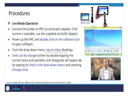
Then this live mode operation is there and through serial port adapter we use either using AC current or battery operation is also possible. Then we can use the tap on View button readings and those units can also be changed depending upon what kind of unit we are needing the values into.
