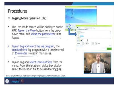
Then if we log into this mode operation basically then we can select the parameters according to the need, and we can also ensure which interval we need to have like per minute or 15 minute those kinds of default values 15 minutes, so, that kind of most of the cases we use 15 minutes otherwise we can change it for per minute or depending upon the need of the data.
