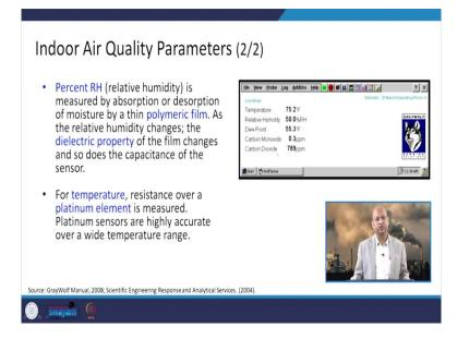
If we talk about like percent relative humidity, so, it is measured by either absorption or desorption methodology of the moisture by a thin polymeric film. So, the relative humidity changes the, this dielectric property of the film also changes. So, according the variation comes in concentration are measured. For temperature basically we use the platinum element which is quite robust to give readings about the temperature. So, this is the way different parameters are used.
