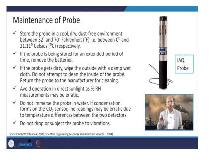
Then, how to maintain or what is the requirement of the maintenance of the probe so that it gives better reading or reliable reading and does not give us the erroneous readings. First of all, we need to store those probes or sensors in a cool, dry and dust free environment the temperature should be less than around 21 degrees Celsius, 21.11 or so.
