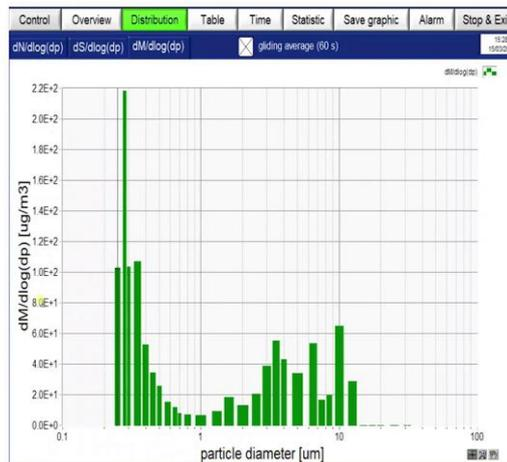
So, coming to the next step that is distribution. In distribution tab you can see a log table is being shown. So, in this first table, that is the log table. You can see the X axis you can see the particle diameter or particle sizes and in Y axis, you can see the this microgram (μg/m<sup>3</sup>)(20:04).
