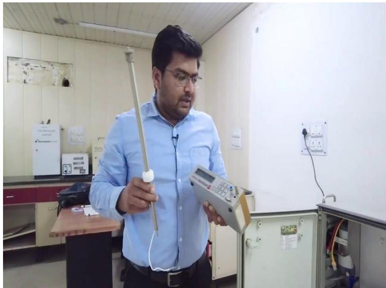
So, this is the spectrometer and this is the front panel of the spectrometer, here you can see this LCD screen where we are seeing the readings of all the PM<sub>10</sub> PM<sub>2.5</sub> all the particles and these are the control buttons, where we are using these buttons we are controlling this spectrometer and this is the sample inlet. So, in this sample inlet this sampling pipe is being fitted in this spectrometer and this spectrometer is being placed in this field housing.
