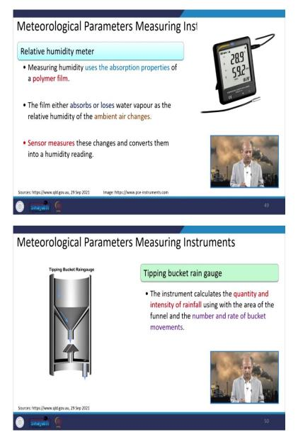
Similarly, you can see these instruments which are measuring like relative humidity and then this for the rainfall intensity you can see, very simple instrument is there. So, in funnel this is stored and then the rate of bucket movements all those play role in measurements of this particular entity of rainfall.
