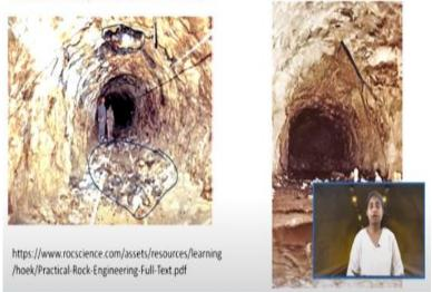
Now, here these 2 pictures give you the idea that, how the upon the excavation the blocks fall under the gravity from the roof, you take a look here in this zone and see how the rock pieces which are fallen. Here, in this case, similarly here on this you see a wedge has already been fallen from this particular part of the excavation.
