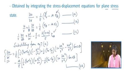
So here we obtain the displacement from the stress displacement equation for plane stress state and integrating these. So, what are these stress displacement equation for plane stress situation. So first, we will take a plane stress situation and then we will also discuss about the plane strain state. So here, we have these equations in the polar coordinate form in this manner that is:
