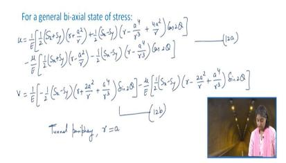
So, this is what is going to be the equation for v, makes it as 11b. Now, let us try to apply the boundary condition to obtain these constants. So, the first boundary condition here is going to be that displacement v will be equal to 0, when  $\theta = 0$  or  $\pi$  by 2 for all values of r. This is due to symmetry so let us substitute C to be equal to 0 at  $\theta = 0$ . What we get is?
